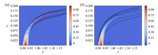
Figure 6. Steady-state solution of the reactive jet in crossflow at z = 0.15. (a) Contours of the fuel mass fraction  $\rho Y_f$  and contour lines of the temperature profile: red, 90 % of the maximum temperature. (b) Contours of the fuel mass fraction  $\rho Y_f$  and density dilatation  $\|\nabla \rho\|$ .
