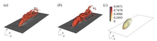
Figure 1. (a,b) Isosurfaces of the Q-criterion as an indicator of vortical structures in the instantaneous flow field. The grey contours depict the streamwise velocity component. (c) The instantaneous scalar field, presented by using volume rendering of the fuel mass density. High values of mass density are coloured in red, lower values in yellow. (a) Non-reactive jet in crossflow. (b) Reactive jet in crossflow. (c) Reacting scalar field.
