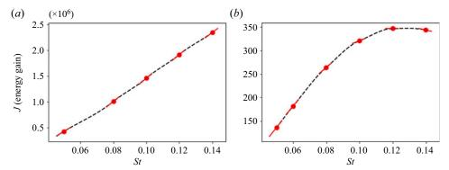
Figure 9. Frequency response of the two configurations: (a) non-reactive jet; (b) reactive jet. Red circles, locations where J and  $dJ/d\omega$  are extracted using the adjoint-based algorithm; solid red line, local gradient; black dashed line, cubic Hermite interpolation.
