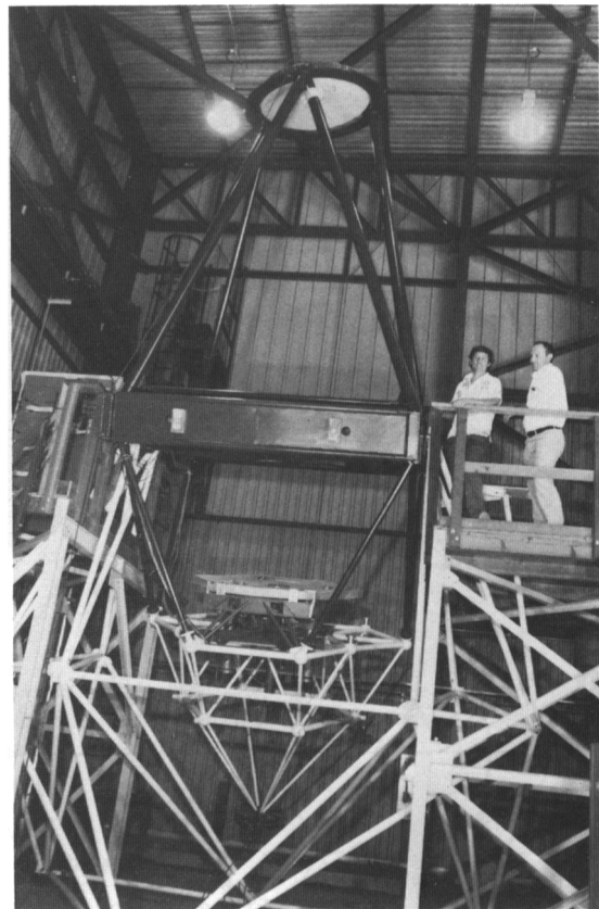
10. Photo of the Technical Demonstration Telescope with concrete optics and the active control system in place.
