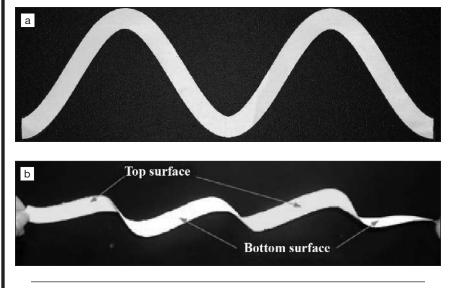
Figure 1. (a) A piece of paper is cut into a serpentine. (b) When pulled, the serpentine elongates by twisting out of plane.
