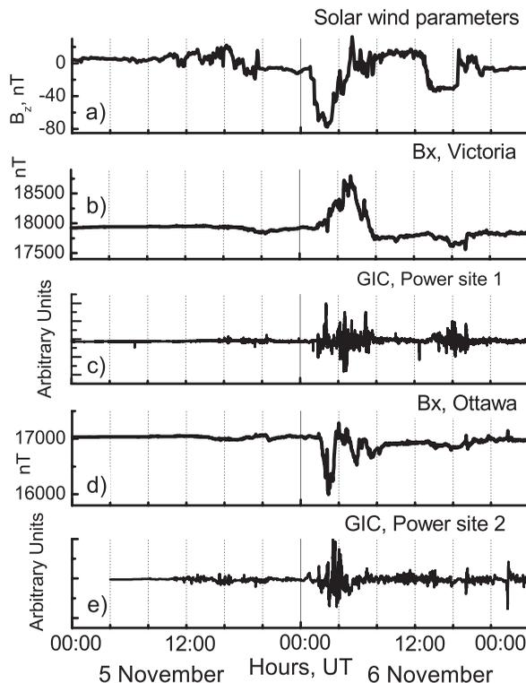
Figure 1. Magnetic field in the solar wind and on the ground and GIC on 5-6 November.
