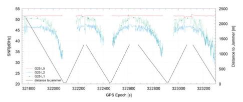
Figure 17. Comparison between L1, L2 and L5 SNR for GPS SV 25.
