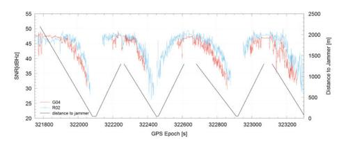
Figure 10. SNR for G04 and R02 (low elevation satellites).
