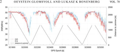
Figure 9. SNR for G25 and R10 (high elevation satellites).
