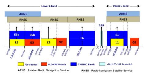
Figure 1. GNSS Frequency allocation (Subirana et al., 2011).
