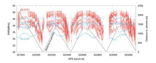
Figure 15. G1 and G2 SNR for GLONASS satellites.
