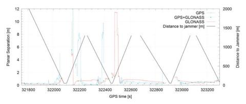
Figure 12. Planar accuracy for DGPS dual frequency solutions.
