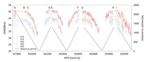
Figure 8. Comparison of SNR for high (G25) and low elevation GPS satellites.
