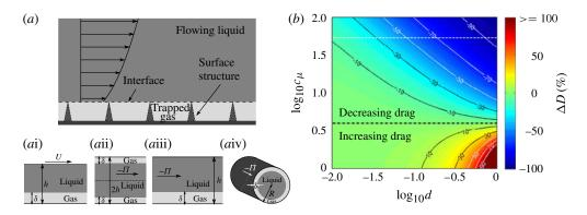
FIGURE 1. (a) Schematics of laminar flow over an idealized superhydrophobic surface, with four flow configurations considered: (ai) Couette flow; (aii) symmetric pressure-driven channel flow; (aiii) one-sided pressure-driven channel flow; and (aiv) pipe flow. (b) Change in drag,  $\Delta D$ , as a function of viscosity ratio ( $c_{\mu}$ ) and lubricant thickness (d), for a laminar Couette flow configuration (ai) with no net mass flow in the lubricant layer (from Busse *et al.* 2013).
