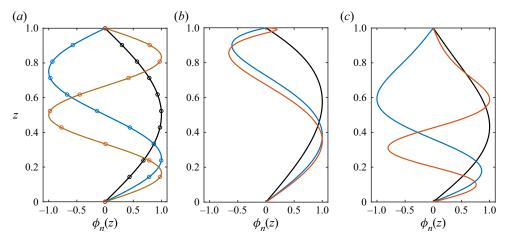
Figure 3. Mode shapes in a uniform stratification with an exponential background velocity profile (3.1) for (a)  $Ri = \infty$  (continuous lines, no shear),  $Ri = 10^5$  (hollow circles, weak shear), (b) Ri = 1 (finite shear, cograde modes) and (c) Ri = 1 (finite shear, retrograde modes). In each panel, mode numbers n = 1 (black), 2 (blue) and 3 (red) are shown.
