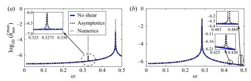
Figure 4. Superharmonic wave amplitude  $\log_{10}[\bar{h}_{mn}^{max}]$  (2.12) plotted as a function of primary wave frequency  $\omega$  at  $Ri=\infty$  (no shear, shown in blue) and  $Ri=10^7$  (asymptotics, numerics), for representative modal interactions specified by (m,n)=(a) (2, 3), (b) (2, 5). The insets show a zoomed-in view of the additional divergences that occur in the presence of weak shear.
