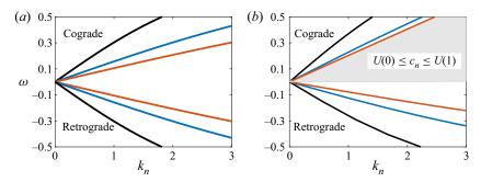
Figure 2. Dispersion curves for different mode numbers in a uniform stratification for (a)  $Ri = \infty$  and (b) Ri = 1. In each panel, the black, blue and red colours correspond to mode numbers n = 1, 2 and 3, respectively.
