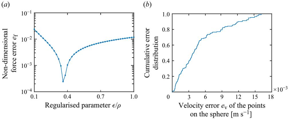
Figure 9. (a) Resistive force error  $e_f$  for two isolated ellipsoids is dependent on the regularised parameter  $\epsilon$ . (b) Cumulative distribution of the velocity error  $e_v$  for the points on the sphere.
