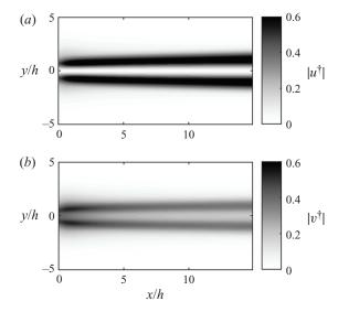
Figure 8. The absolute value of the streamwise (*a*) and transversal (*b*) velocity component of the most unstable adjoint mode.
