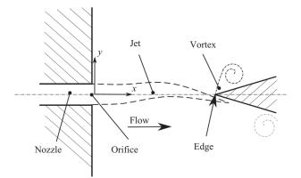
Figure 1. The schematic drawing of the edge tone.
