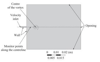
Figure 4. The CFD configuration and boundary conditions of the excited plane jet.
