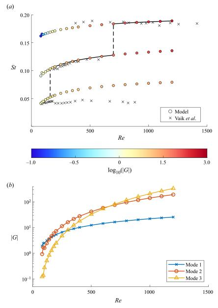
Figure 13. (a) The comparison of the oscillation frequencies predicted by the model with the measurements of Vaik *et al.* (2014*a*). The bluish circles indicate gains below one, i.e. no oscillation is generated there. (b) The absolute open loop gain of the calculated modes. Parabolic inlet velocity profile, nozzle–edge distance relative to the nozzle height is 9.72.
