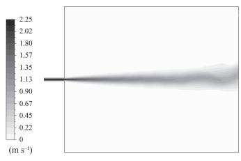
Figure 6. The velocity field of the simulation at t = 0.4 s in the case of the modified potential vortex.
