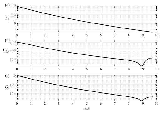
Figure 12. Parts of the feedback loop as the function of the streamwise coordinate:  $K_i$ , downstream amplification;  $C_{0,i}$ , amplitude of the instability waves triggered by the forcing of the edge;  $G_i$ , local total gain. Parabolic inlet velocity profile, St = 0.1145, Re = 300.
