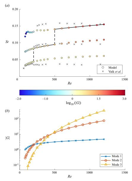
Figure 14. (a) The comparison of the oscillation frequencies predicted by the model with the measurements of Vaik *et al.* (2014*a*). The bluish circles indicate gains below one, i.e. no oscillation is generated there. (b) The absolute open loop gain of the calculated modes. Top-hat inlet velocity profile, nozzle–edge distance relative to the nozzle height is 10.26.
