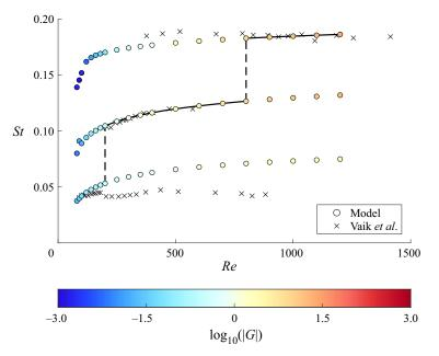
Figure 15. The comparison of the oscillation frequencies predicted by the model with the measurements of Vaik *et al.* (2014*a*). Modified incompressible dipole forcing field ( $r_0 = 0.1, L = 0.5h$ ), parabolic inlet velocity profile. The bluish circles indicate gains below one, i.e. no oscillation is generated there.
