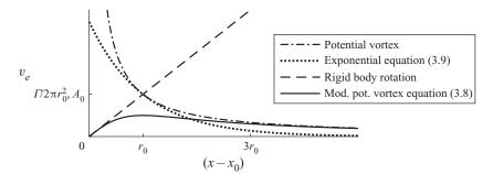
Figure 3. The velocity field of various vortex formulae.
