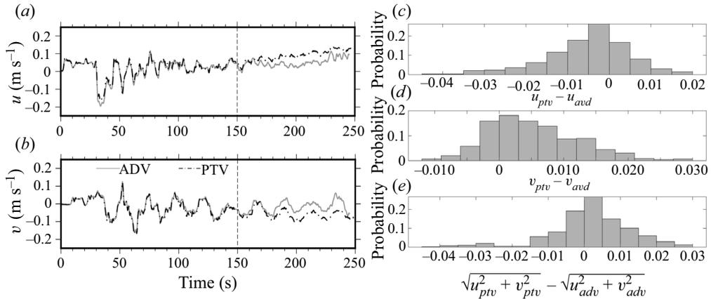
Figure 9. (a,b) Comparison between horizontal velocities extracted from the ADV (located at  $x = 4.52$  m,  $y = 0.01$  m,  $z = 0.271$  m) and the corresponding velocities extracted from PTV analysis – values sampled at 3 Hz. (c–e) Statistics for the differences between the two data-sets corresponding to the time interval  $0 \leq t \leq 150$  s.
