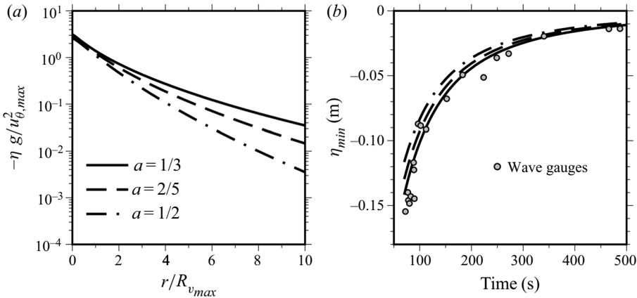
Figure 14. Evolution of the TCS free surface. (a) Normalised FSE profiles for different  $a$ -profiles. (b) Evolution of the free surface at the TCS-centre (minimum) as recorded by the closest wave gauge (grey points) and as predicted by (4.9) for different  $a$ -profiles. Note that  $\eta_{\min}$  is independent of  $R_{v_{\max}}$ .
