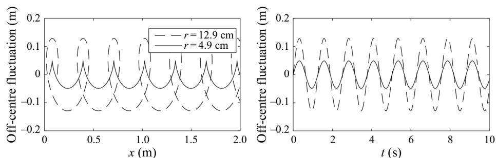
Figure 18. Paths of off-centre tracers in an idealised shielded-Gaussian vortex flow with  $\omega_0 = 10 \text{ s}^{-1}$ ,  $R = 1 \text{ m}$ , and vortex-centre translation velocity  $u = 0.25 \text{ m s}^{-1}$ .
