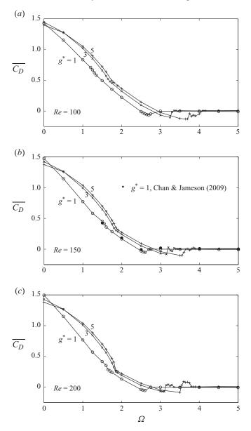
FIGURE 11. (a)–(c) Flow past a doublet-like counter-rotating cylinder: numerically determined time-averaged values of the drag coefficient (upper cylinder).
