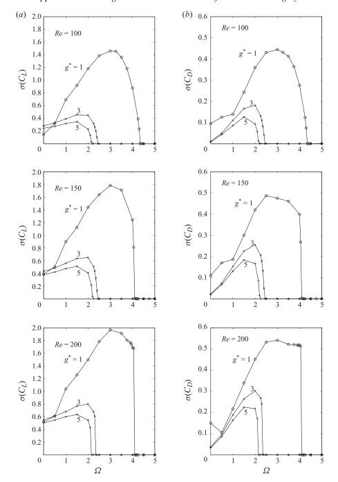
FIGURE 22. Flow past a reverse doublet-like counter-rotating configuration: the standard deviation of coefficients of lift (a) and drag (b).
