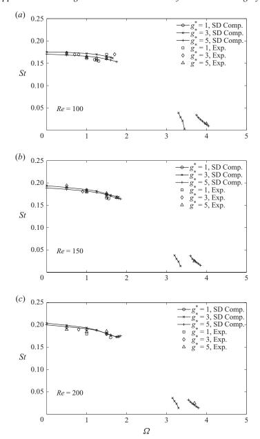
FIGURE 14. (a)–(c) Flow past a doublet-like counter-rotating cylinder: numerically determined Strouhal number (anti-phase shedding only).
