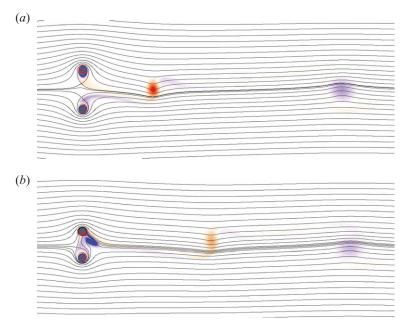
FIGURE 24. Instantaneous streamlines and vorticity for the second instability of the doublet-like counter-rotating configuration (computational results): (a) Re = 200,  $g^* = 5$ ,  $\Omega = 3.75$ ; (b) Re = 200,  $g^* = 3$ ,  $\Omega = 3.25$ . Vorticity contour levels are -0.1 (blue) and 0.1 (red).
