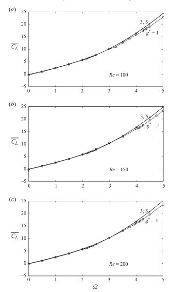
FIGURE 18. (a)–(c) Flow past a reverse doublet-like counter-rotating cylinder: numerically determined time-averaged values of lift coefficient (lower cylinder).
