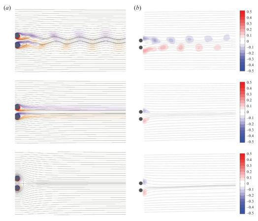
FIGURE 7. Doublet-like rotational configuration: streamlines and vorticity at various rotational speeds for  $g^*=1$ , Re=100. (a) Computational results. (b) Experimental results. First row,  $\Omega=1.2$ ; second row,  $\Omega=1.5$ ; third row  $\Omega=3$ . For this case,  $\Omega_{crit}=1.35$  (computational) and 1.4 (experimental). Vorticity contour levels for the computational and experimental results are the same.
