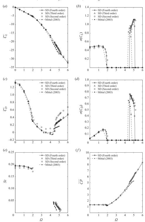
FIGURE 29. Flow past a rotating circular cylinder: mean  $C_L$  (a), standard deviation of  $C_L$  (b), mean  $C_D$  (c), standard deviation of  $C_D$  (d),  $S_T$  (e) and mean  $C_T$  (f).
