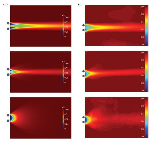
FIGURE 12. Doublet-like rotational configuration: normalized streamwise velocity contours at various rotational speeds for  $g^* = 1$ , Re = 100. (a) Computational results. (b) Experimental results. First row,  $\Omega = 1.5$ ; second row,  $\Omega = 2$ ; third row,  $\Omega = 4$ .
