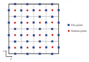
FIGURE 3. (Colour online) Distribution of flux and solution points for the fourth-order SD scheme.
