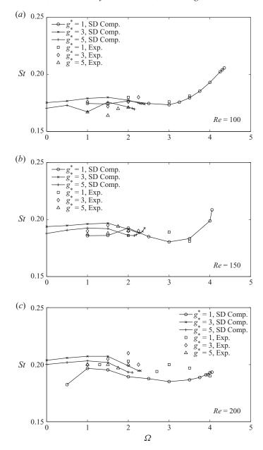
FIGURE 20. (a)–(c) Flow past a reverse doublet-like counter-rotating cylinder: numerically determined Strouhal number (anti-phase shedding only).
