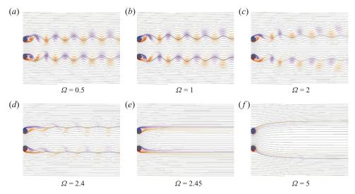
FIGURE 17. (a)–(f) Instantaneous streamlines and vorticity for reverse doublet-like counter-rotating cylinder (computational results): Re = 150,  $g^* = 3$ . Vorticity contour levels are -0.5 (blue) and 0.5 (red).
