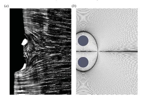
FIGURE 9. (Colour online) Experimental streaklines (a) and computational streamlines (b) showing the existence of the stagnation point and virtual elliptical body for the doublet-like rotational configuration:  $g^* = 1$ , Re = 150,  $\Omega = 3.1$ .
