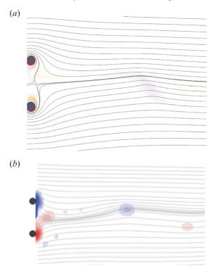
FIGURE 25. Instantaneous streamlines and vorticity for the second instability of the doublet-like counter-rotating configuration, Re = 100,  $g^* = 5$ ,  $\Omega = 4$ : (a) computational; (b) experimental. Vorticity contour levels are -0.5 (blue) and 0.5 (red).
