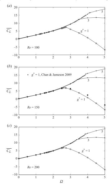
FIGURE 10. (a)–(c) Flow past a doublet-like counter-rotating cylinder: numerically determined time-averaged values of the lift coefficient (upper cylinder).
