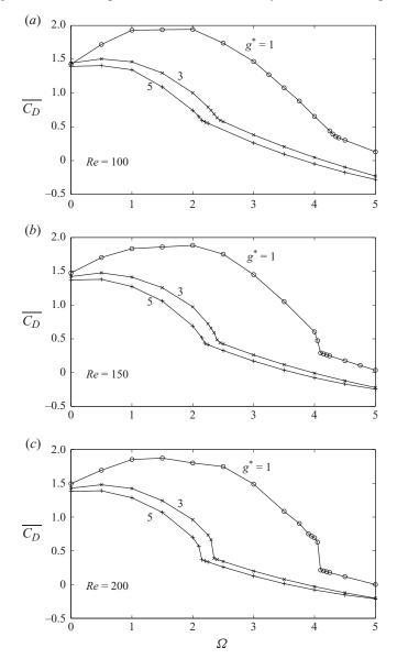
FIGURE 19. (a)—(c) Flow past a reverse doublet-like counter-rotating cylinder: numerically determined time-averaged values of drag coefficient (lower cylinder).
