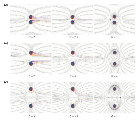
FIGURE 8. Instantaneous streamlines and vorticity showing the evolution of virtual elliptical body for the doublet-like configuration (computational results). (a)  $g^* = 1$ , Re = 150; (b)  $g^* = 3$ , Re = 150; (c)  $g^* = 5$ , Re = 150. Stagnation points are represented by ' $\bullet$ '. Vorticity contour levels are -0.5 (blue) and 0.5 (red).
