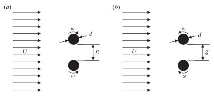
FIGURE 2. Counter-rotating circular cylinder pair. (a) Doublet-like configuration. (b) Reverse doublet-like configuration.
