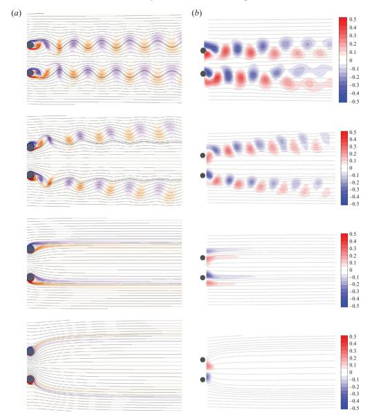
FIGURE 15. Reverse doublet-like rotational configuration: streamlines and vorticity at various rotational speeds for  $g^*=3$ , Re=200. (a) Computational results. (b) Experimental results. First row,  $\Omega=0$ ; second row,  $\Omega=2$ ; third row,  $\Omega=2.4$ ; fourth row,  $\Omega=5$ . Vorticity contour levels for the computational and experimental results are the same.
