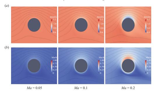
FIGURE 30. Flow past a single rotating circular cylinder, Re = 200,  $\omega = 3\Omega$ : normalized density (a) and Mach (b) contours at different free stream Mach numbers.
