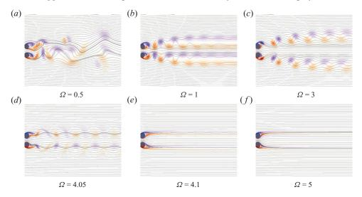
FIGURE 16. (a)—(f) Instantaneous streamlines and vorticity for reverse doublet-like counter-rotating cylinder (computational results): Re = 150,  $g^* = 1$ . Vorticity contour levels are -0.5 (blue) and 0.5 (red).
