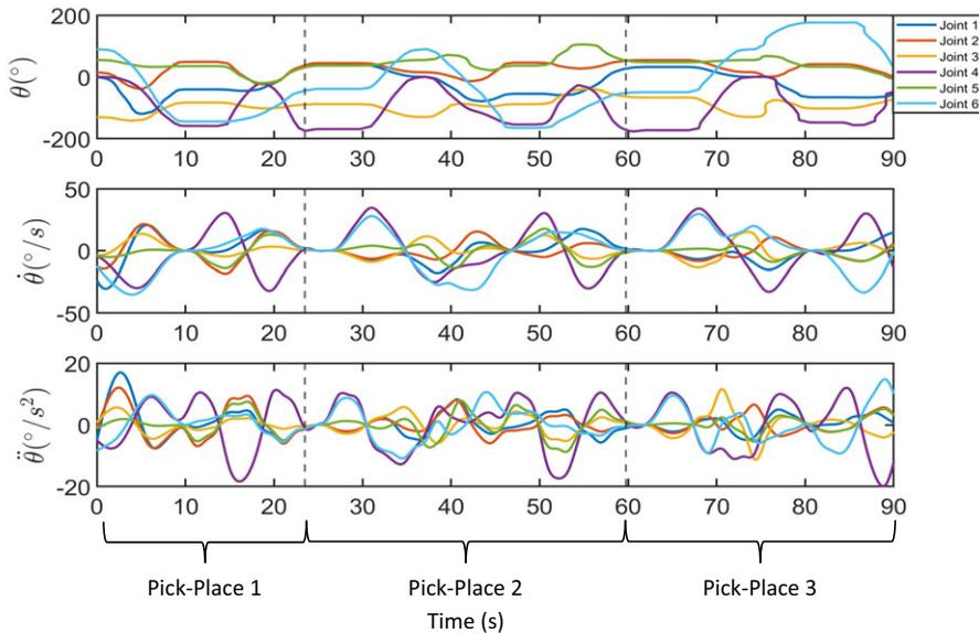
**Figure 8.** Motion profile for a randomly selected bin-picking scenario with the Kinova Gen3 robotic arm. **top row:** joints angles plot **middle row:** joints velocities plot **bottom row:** joints accelerations plot.
