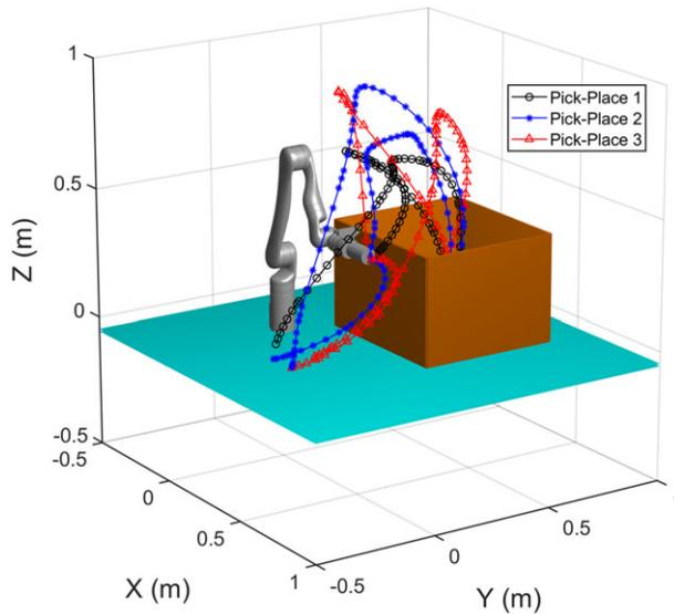
**Figure 7.** Cartesian space path for a randomly selected bin-picking scenario with the Kinova Gen3 robotic arm. In this scenario, the robot should pick three different objects and place them on the table.
