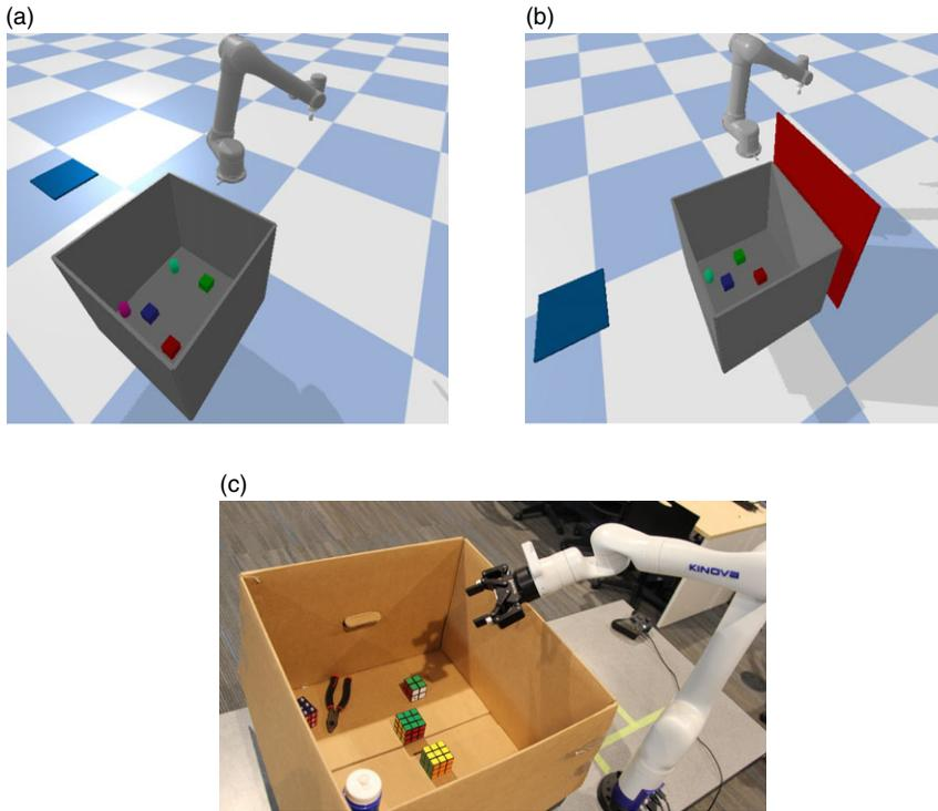
**Figure 5.** Experimental environments: (a) UR5 scene, (b) UR5 scene with a wall as an obstacle, (c) Real-world implementation on Kinova Gen3.
