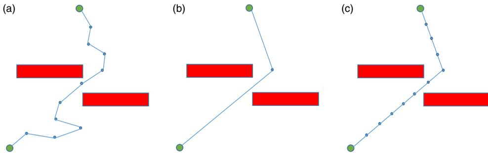
**Figure 4.** Post-processing procedure: (a) The generated path by the planner, (b) Path after binary state contraction, (c) Path after resampling.
