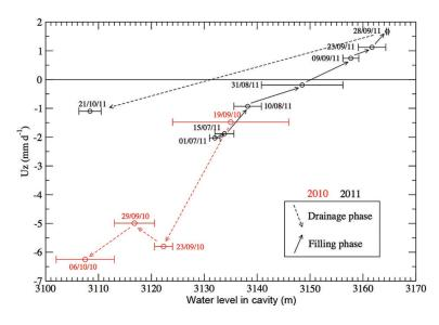
**Fig. 7.** Mean vertical ice flow velocities measured in the vicinity of the cavity after pumping and during the refilling. In 2011 the bottom of the cavity was filled with ice coming from the roof collapse, which explains the different behavior below 3130 m and a similar behavior above. Date format is dd/mm/yy.
