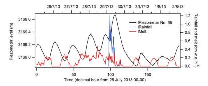
Fig. 13. Changes in water level recorded at piezometer No. 65, melt and rainfall from 25 July to 2 August 2013. Date format is dd/mm/yy.
