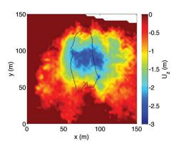
**Fig. 6.** Vertical displacements from August 2010 to August 2011 derived from DEMs obtained in 2007 and 2011. The DEM difference was corrected for the ice ablation measured over this period. The black solid line shows the location of the cavern obtained from sonar measurements.
