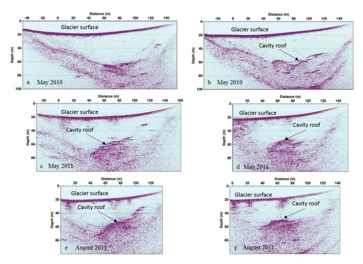
Fig. 4. Evolution of the two transverse profiles shown in Figure 1 between May 2010 and August 2011. Cross sections (a), (c) and (e) are located downstream of cross sections (b), (d) and (f).
