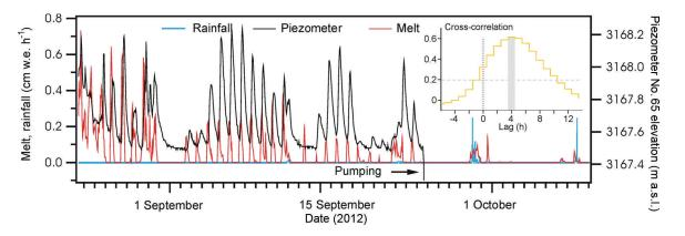
Fig. 12. Relationship between water level of the cavity, melt and rainfall from 24 August to 10 October 2012. The cross-correlation between melt rate and deferred cavity-filling rate as a function of the time lag is reported in the inset. The dashed line is the significance threshold.
