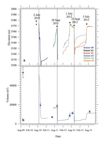
**Fig. 2.** (a) Water levels measured in the boreholes between 2010 and 2013. (b) Evolution of the volume of water within the cavity between 2009 and 2013 as determined by the volume of pumped water and modeled surface meltwater. The blue circles indicate volumes measured by the 3-D SNMR method (Legchenko and others, 2014). The vertical dashed lines correspond to the beginning of successive pumping operations.
