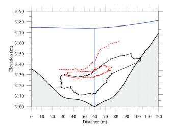
**Fig. 5.** Cross section of the glacier with the surface (blue) and bedrock (gray). The geometry of the cavity obtained from sonar measurements carried out on 1 September 2010 and 23 September 2011 is plotted in black and red solid lines respectively. The dashed lines correspond to the roof of the cavity obtained from GPR measurements in May 2010. The vertical blue line is the borehole from which the sonar measurements were performed.
