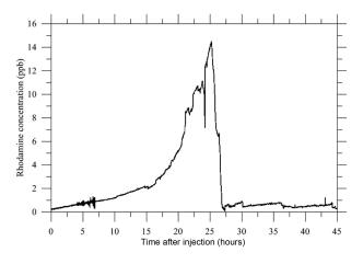
**Fig. 11.** Dye tracing with 30 s time-step data since 28 September 2012 at 11:00 LT. The dye was injected at 12:00 LT. The dye concentration in the pumping water at the fluorometer is expressed in ppb and the detection threshold is 1 ppb.
