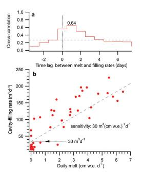
**Fig. 10.** Relation between melt and filling daily rates in 2011 (excluding rainfall days). (a) Cross-correlation between melt rate and deferred cavity-filling rate as a function of the time lag; the dashed line is the significance threshold. (b) Linear correlation between filling rate and melting at day +1 for the days without precipitation. The intercept is the filling rate expected without melting. The sensitivity is equivalent to an effective draining surface area of  $3000 \text{ m}^2$ .
