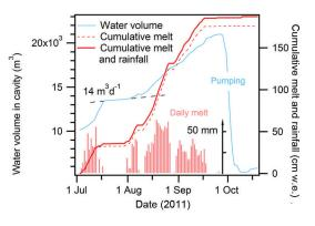
**Fig. 9.** Water volume in 2011 as reconstructed from water level, pumping and SNMR data (blue line), and cumulative melt given by the SEB (dashed line), including rainfall (red line). Bars are daily melt on a mm scale. The slope of  $14 \text{ m}^3 \text{ d}^{-1}$  reveals the daily filling runoff observed between 18 and 31 July without surface melting.
