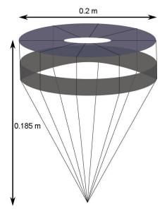
Fig. 6. Disk Gap Band parachute design.
