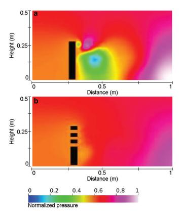
**Fig. 4.** Results of finite-element modelling the aerodynamics of components of ADIOS. Normalized air pressure around (a) a solid snow brake and (b) a geometrically porous snow brake. The direction of airflow was left to right.
