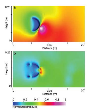
**Fig. 7.** Results of finite-element modelling the aerodynamics of components of ADIOS. Normalized air pressure around (a) a solid flat circular parachute and (b) a Disk Gap Band parachute. The direction of airflow was left to right.
