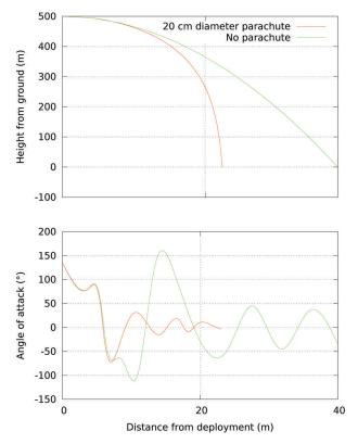
Fig. 5. Device trajectory and stability data from experiments.
