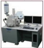
feature low vacuum observation method (6 - 270Pa), which enables observation of non-conductive samples like electronic components, and water containing samples such as cultured cells, without any sample preparation.
