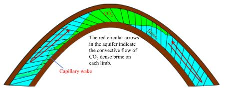
Figure 8. Diagram illustrating a possible pattern for the migration of a plume of buoyant injectate (green fluid) in a cross-bedded anticline initially saturated with saline aqueous solution (blue fluid), in the case that the buoyancy forces dominate the flow of the injectate. If the flow of  $CO_2$  is buoyancy dominated, this figure identifies that different patterns of ascent and of capillary trapping may arise depending on the bedding.
