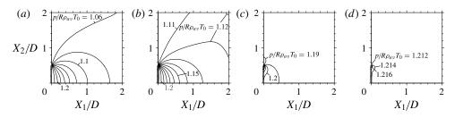
FIGURE 7. Isolines of the pressure for the thermal edge flow  $(T_w^+/T_0 = T_w^-/T_0 = 2 \text{ and } L/D = 4)$ . (a)  $Kn = 5 (p/R\rho_{av}T_0 = 1.06 + 0.01m; m = 0, ..., 8)$ , (b)  $Kn = 0.5 (p/R\rho_{av}T_0 = 1.11 + 0.005m; m = 0, ..., 12)$ , (c)  $Kn = 0.05 (p/R\rho_{av}T_0 = 1.19 + 0.005m; m = 0, ..., 8)$ , (d)  $Kn = 0.01 (p/R\rho_{av}T_0 = 1.212 + 0.002m; m = 0, 1, ..., 9)$ .
