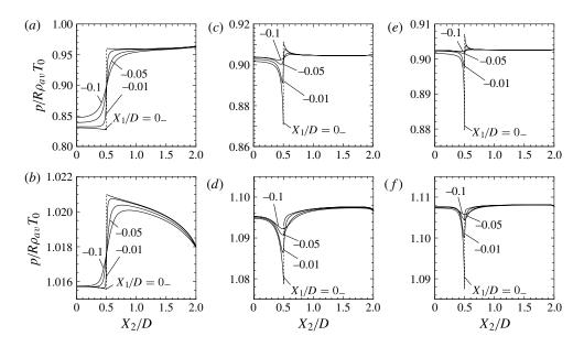
FIGURE 19. As in figure 17, but for the pressure p: (a,b) Kn = 5; (c,d) Kn = 0.05; (e,f) Kn = 0.02.
