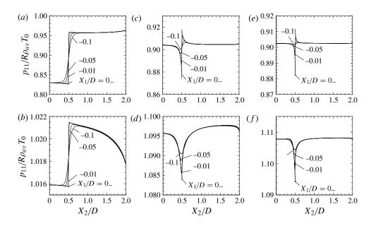
FIGURE 24. Distributions of the stress  $p_{11}$  along four lines  $X_1/D = 0_-$ , -0.01, -0.05 and -0.1 close to the plate for various Kn (L/D = 4). Top row (a,c,e) Thermal edge flow around a cooled plate ( $T_w^+/T_0 = T_w^-/T_0 = 0.5$ ); bottom row (b,d,f) radiometric flow ( $T_w^+/T_0 = 2$  and  $T_w^-/T_0 = 1$ ): (a,b) Kn = 5; (c,d) Kn = 0.05; (e,f) Kn = 0.02.
