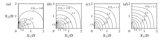
FIGURE 6. Isolines of the temperature for the thermal edge flow  $(T_w^+/T_0 = T_w^-/T_0 = 2$ and L/D = 4). (a) Kn = 5  $(T/T_0 = 1.05 + 0.05m; m = 0, 1, ..., 8)$ , (b) Kn = 0.5  $(T/T_0 = 1.05 + 0.05m; m = 0, 1, ..., 12)$ , (c) Kn = 0.05  $(T/T_0 = 1.1 + 0.1m; m = 0, 1, ..., 8)$ , (d) Kn = 0.01  $(T/T_0 = 1.1 + 0.1m; m = 0, 1, ..., 8)$ .
