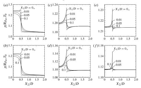
FIGURE 16. As in figure 14, but for the pressure p: (a,b) Kn = 5; (c,d) Kn = 0.05;(*e*,*f*) Kn = 0.01.
