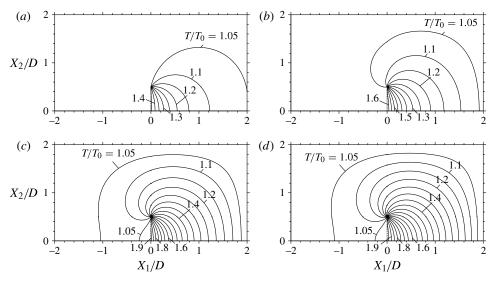
FIGURE 12. Isolines of the temperature for the radiometric flow  $(T_w^+/T_0 = 2, T_w^-/T_0 = 1)$ and L/D = 4. (a) Kn = 5  $(T/T_0 = 1.05 + 0.05m; m = 0, 1, ..., 8)$ , (b) Kn = 0.5  $(T/T_0 = 1.05 + 0.05m; m = 0, 1, ..., 11)$ , (c) Kn = 0.05  $(T/T_0 = 1.05 + 0.05m; m = 0, 1, ..., 17)$ , (d) Kn = 0.01  $(T/T_0 = 1.05 + 0.05m; m = 0, 1, ..., 18)$ .
