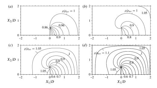
FIGURE 11. Isolines of the density for the radiometric flow  $(T_w^+/T_0 = 2, T_w^-/T_0 = 1 \text{ and } L/D = 4)$ . (a) Kn = 5  $(\rho/\rho_{av} = 0.84 + 0.02m; m = 0, 1, ..., 8)$ , (b) Kn = 0.5  $(\rho/\rho_{av} = 0.75 + 0.05m; m = 0, 1, ..., 6)$ , (c) Kn = 0.05  $(\rho/\rho_{av} = 0.6 + 0.05m; m = 0, 1, ..., 9)$ , (d) Kn = 0.01  $(\rho/\rho_{av} = 0.6 + 0.05m; m = 0, 1, ..., 9)$ .
