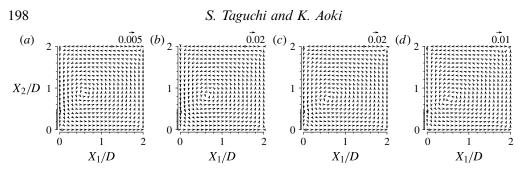
FIGURE 2. Thermal edge flow  $(T_w^+/T_0 = T_w^-/T_0 = 2 \text{ and } L/D = 4)$ . (a) Kn = 5, (b) Kn = 0.5, (c) Kn = 0.05, (d) Kn = 0.01. The arrows indicate the flow velocity vector  $(v_1, v_2)/(2RT_0)^{1/2}$  at its starting point. The reference length is shown above each plot.
