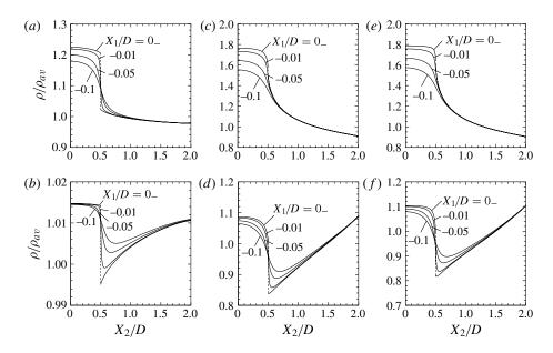
FIGURE 17. Distributions of the density  $\rho$  along four lines  $X_1/D = 0_-$ , -0.01, -0.05 and -0.1 close to the plate for various Kn (L/D = 4). Top row (a,c,e) Thermal edge flow around a cooled plate ( $T_w^+/T_0 = T_w^-/T_0 = 0.5$ ); bottom row (b,d,f) radiometric flow ( $T_w^+/T_0 = 2$  and  $T_w^-/T_0 = 1$ ): (a,b) Kn = 5; (c,d) Kn = 0.05; (e,f) Kn = 0.02.
