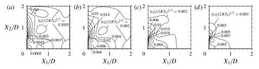
FIGURE 4. Isolines of the flow speed  $|v_i| = (v_1^2 + v_2^2)^{1/2}$  for the thermal edge flow  $(T_w^+/T_0 = T_w^-/T_0 = 2 \text{ and } L/D = 4)$ . (a)  $Kn = 5 (|v_i|/(2RT_0)^{1/2} = 0.0005m; m = 1, 2, ..., 9)$ , (b)  $Kn = 0.5 (|v_i|/(2RT_0)^{1/2} = 0.002m; m = 1, 2, ..., 10)$ , (c)  $Kn = 0.05 (|v_i|/(2RT_0)^{1/2} = 0.002m; m = 1, 2, ..., 8)$ .
