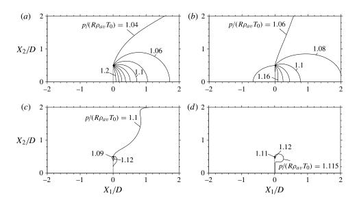
FIGURE 13. Isolines of the pressure for the radiometric flow  $(T_w^+/T_0 = 2, T_1/T_0 = 2 \text{ and } L/D = 4)$ . (a)  $Kn = 5 (p/R\rho_{av}T_0 = 1.04 + 0.02m; m = 0, ..., 8)$ , (b)  $Kn = 0.5 (p/R\rho_{av}T_0 = 1.04 + 0.02m; m = 0, ..., 7)$ , (c)  $Kn = 0.05 (p/R\rho_{av}T_0 = 1.09 + 0.01m; m = 0, ..., 5)$ , (d)  $Kn = 0.01 (p/R\rho_{av}T_0 = 1.095 + 0.005m; m = 0, 1, ..., 10)$ .
