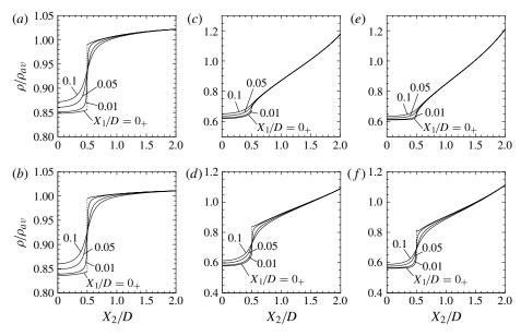
FIGURE 14. Distributions of the density  $\rho$  along four lines  $X_1/D = 0_+$ , 0.01, 0.05 and 0.1 close to the plate for various Kn (L/D = 4). Top row (a,c,e) Thermal edge flow around a heated plate ( $T_w^+/T_0 = T_w^-/T_0 = 2$ ); bottom row (b,d,f) radiometric flow ( $T_w^+/T_0 = 2$  and  $T_w^-/T_0 = 1$ ): (a,b) Kn = 5; (c,d) Kn = 0.05; (e,f) Kn = 0.01.
