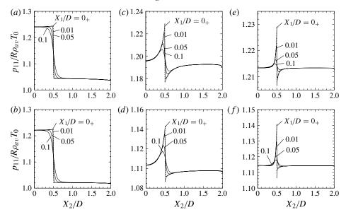
FIGURE 23. Distributions of the stress  $p_{11}$  along four lines  $X_1/D = 0_+$ , 0.01, 0.05 and 0.1 close to the plate for various Kn (L/D = 4). Top row (a,c,e) Thermal edge flow around a heated plate ( $T_w^+/T_0 = T_w^-/T_0 = 2$ ); bottom row (b,d,f) radiometric flow ( $T_w^+/T_0 = 2$  and  $T_w^-/T_0 = 1$ ): (a,b) Kn = 5; (c,d) Kn = 0.05; (e,f) Kn = 0.01.
