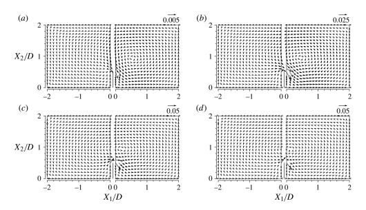
FIGURE 8. Radiometric flow  $(T_w^+/T_0 = 2, T_w^-/T_0 = 1 \text{ and } L/D = 4)$ . (a) Kn = 5, (b) Kn = 0.5, (c) Kn = 0.05, (d) Kn = 0.01. The flow fields for  $X_1 \ge 0$  are shown separately. For more details see the caption of figure 2.
