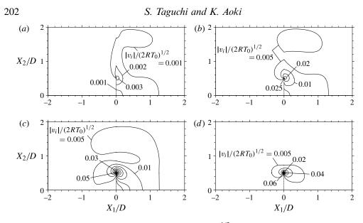
FIGURE 10. Isolines of the flow speed  $|v_i| = (v_1^2 + v_2^2)^{1/2}$  for the radiometric flow  $(T_w^+/T_0 = 2, T_w^-/T_0 = 1 \text{ and } L/D = 4)$ . (a)  $Kn = 5 (|v_i|/(2RT_0)^{1/2} = 0.001m; m = 1, 2, ..., 3)$ , (b)  $Kn = 0.5 (|v_i|/(2RT_0)^{1/2} = 0.005m; m = 1, 2, ..., 5)$ , (c)  $Kn = 0.05 (|v_i|/(2RT_0)^{1/2} = 0.005m; m = 1, 2, ..., 11)$ , (d)  $Kn = 0.01 (|v_i|/(2RT_0)^{1/2} = 0.005m; m = 1, 2, ..., 12)$ . The dashed line indicates the plate.
