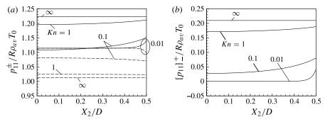
FIGURE 26. (a) Distributions of the normal stress,  $p_{11}^+ = p_{11}(X_1, X_2)|_{X_1/D=0_+}$  and  $p_{11}^- = p_{11}(X_1, X_2)|_{X_1/D=0_-}$ , along each side of the plate and (b) the difference  $[p_{11}]_-^+ = p_{11}^+ - p_{11}^-$  in the radiometric flow  $(T_w^+/T_0 = 2, T_w^-/T_0 = 1 \text{ and } L/D = 4)$ . In (a), the solid line represents  $p_{11}^+$  and the dashed line  $p_{11}^-$ .
