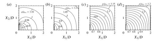
FIGURE 5. Isolines of the density for the thermal edge flow  $(T_w^+/T_0 = T_w^-/T_0 = 2 \text{ and } L/D = 4)$ . (a)  $Kn = 5 (\rho/\rho_{av} = 0.86 + 0.02m; m = 0, 1, ..., 8)$ , (b)  $Kn = 0.5 (\rho/\rho_{av} = 0.75 + 0.05m; m = 0, 1, ..., 7)$ , (c)  $Kn = 0.05 (\rho/\rho_{av} = 0.65 + 0.05m; m = 0, 1, ..., 10)$ , (d)  $Kn = 0.01 (\rho/\rho_{av} = 0.65 + 0.05m; m = 0, 1, ..., 11)$ .
