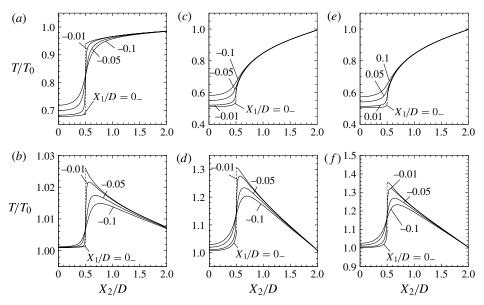
FIGURE 18. As in figure 17, but for the temperature T: (a,b) Kn = 5; (c,d) Kn = 0.05; (e,f) Kn = 0.02.
