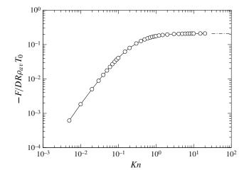
FIGURE 27. Radiometric force *F* versus *Kn* in the case of  $T_w^+/T_0 = 2$  and  $T_w^-/T_0 = 1$  (*L*/*D* = 4). The symbols represents the numerical results which are connected by solid lines. The dash-dotted line indicates the limiting value  $F/DR\rho_{av}T_0 \rightarrow -0.20986$  as  $Kn \rightarrow \infty$ .
