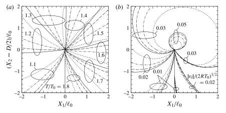
FIGURE 22. Distributions of the temperature *T* and flow speed  $|v_i| = (v_1^2 + v_2^2)^{1/2}$  near the edge for various  $Kn \ (T_w^+/T_0 = 2, \ T_w^-/T_0 = 1 \text{ and } L/D = 4)$ . (a) *T*, (b)  $|v_i|$ . The solid line represents the isoline for Kn = 0.005, the dashed line for Kn = 0.01, the dash-dotted line for Kn = 0.02 and the dotted line for Kn = 0.04.
