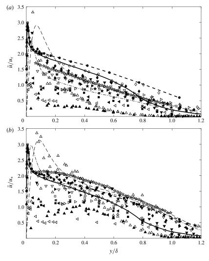
FIGURE 1. Streamwise turbulence intensities in (a) classical outer scaling and (b) transformed according to Morkovin. —,  $\bigcirc$  Klebanoff (1955), ---,  $\bigcirc$  DeGraaff & Eaton (2000), Ma = 0, ---, Priebe & Martin (2011), Ma = 7.2, ---- Duan *et al.* (2011*a*) at Ma = 7.7; other symbols as in table 1. Mach numbers range up to 11.
