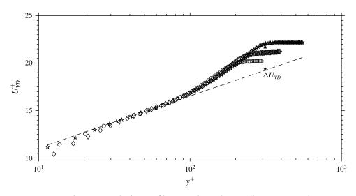
FIGURE 9. Mean velocity profiles transformed according to van Driest. ---: equation (1.2) with  $\kappa = 0.4$  and B = 5.1.
