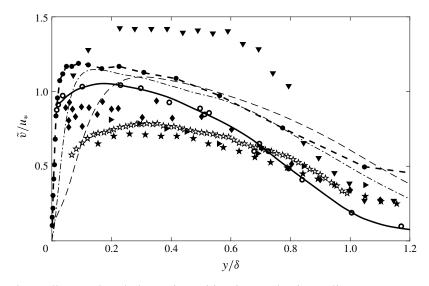
FIGURE 2. Wall-normal turbulence intensities in Morkovin scaling. —,  $\bigcirc$  Klebanoff (1955), ---,  $\bullet$  DeGraaff & Eaton (2000), Ma = 0, ---, Priebe & Martin (2011), Ma = 7.2, ---- Duan *et al.* (2011*a*) at Ma = 7.7; other symbols as in table 1. Mach numbers of experimental data are less than 5.
