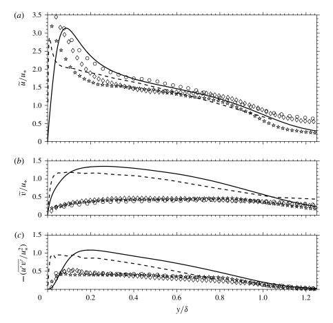
FIGURE 10. Turbulence profiles in outer layer Morkovin scaling. (a) Streamwise and (b) wall-normal velocity r.m.s. (c) Reynolds shear stress. Symbols as in table 6. —, DNS by Priebe & Martin (2011) (Ma = 7.2,  $Re_{\theta} = 3300$ ,  $T_w/T_r = 0.53$ ); ---, DeGraaff & Eaton (2000) (Ma = 0,  $Re_{\theta} = 5200$ ).
