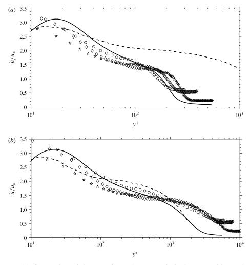
FIGURE 11. Streamwise turbulence scalings. The r.m.s. velocity is presented in Morkovin scaling, as in figure 10. The wall-normal coordinate is presented in (a) inner; (b) semilocal scaling. Lines and symbols as in figure 10.
