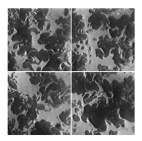
FIGURE 7. Montage of flow visualizations in a plane parallel to the wall at  $y/\delta = 0.77$ . Flow is from left to right. The field of view in each image is 2.0 $\delta$  across the flow and 2.0 $\delta$  in the flow direction. From Baumgartner *et al.* (1997).
