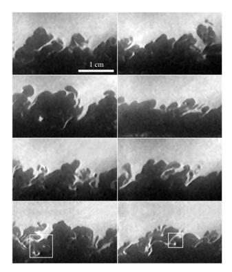
FIGURE 6. Montage of flow visualizations in a plane perpendicular to the wall. Flow is from left to right and the wall is at the bottom of each image. The field of view is  $1.5\delta$  in the wall-normal direction and  $2.5\delta$  in the flow direction. From Baumgartner *et al.* (1997).
