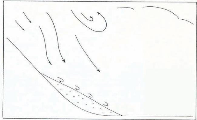
Fig. 11. Schematic view of the positions of the vortices within the kink zone.
