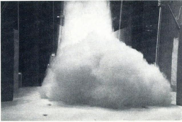
Fig. 4. The side walls of the run-out zone may be removed, thus allowing sideways spreading of the avalanche. (Photograph by F. Hermann.)
