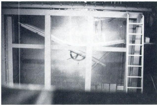
Fig. 2. A general view of the water tank with the submerged chute, kink zone and run-out zone. The ladder gives an estimate of its size. (Photograph by F. Hermann.)
