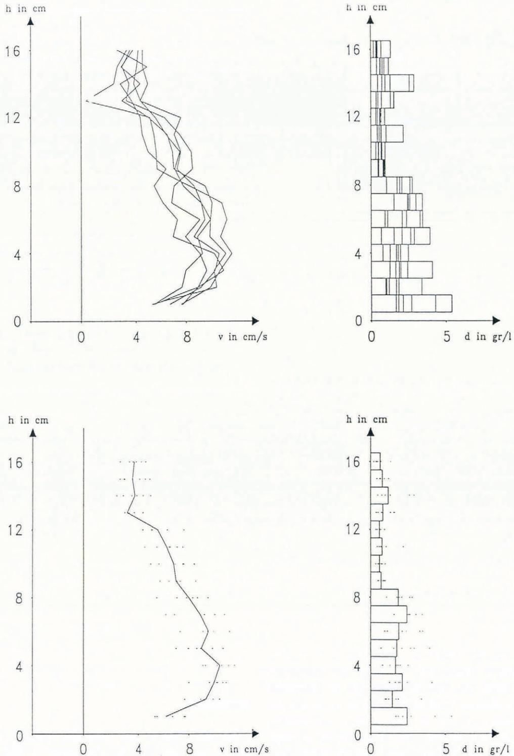
Fig. 7. Single profile measurements (top) and their ensemble average (bottom) of velocity (left) and density (right). Ensemble averaging of seven single experiments turned out to be sufficient to eliminate individual turbulence eddy effects. The parameters of these measurements are  $\alpha = 40^\circ$ ,  $\beta = 55^\circ$  in position B.
