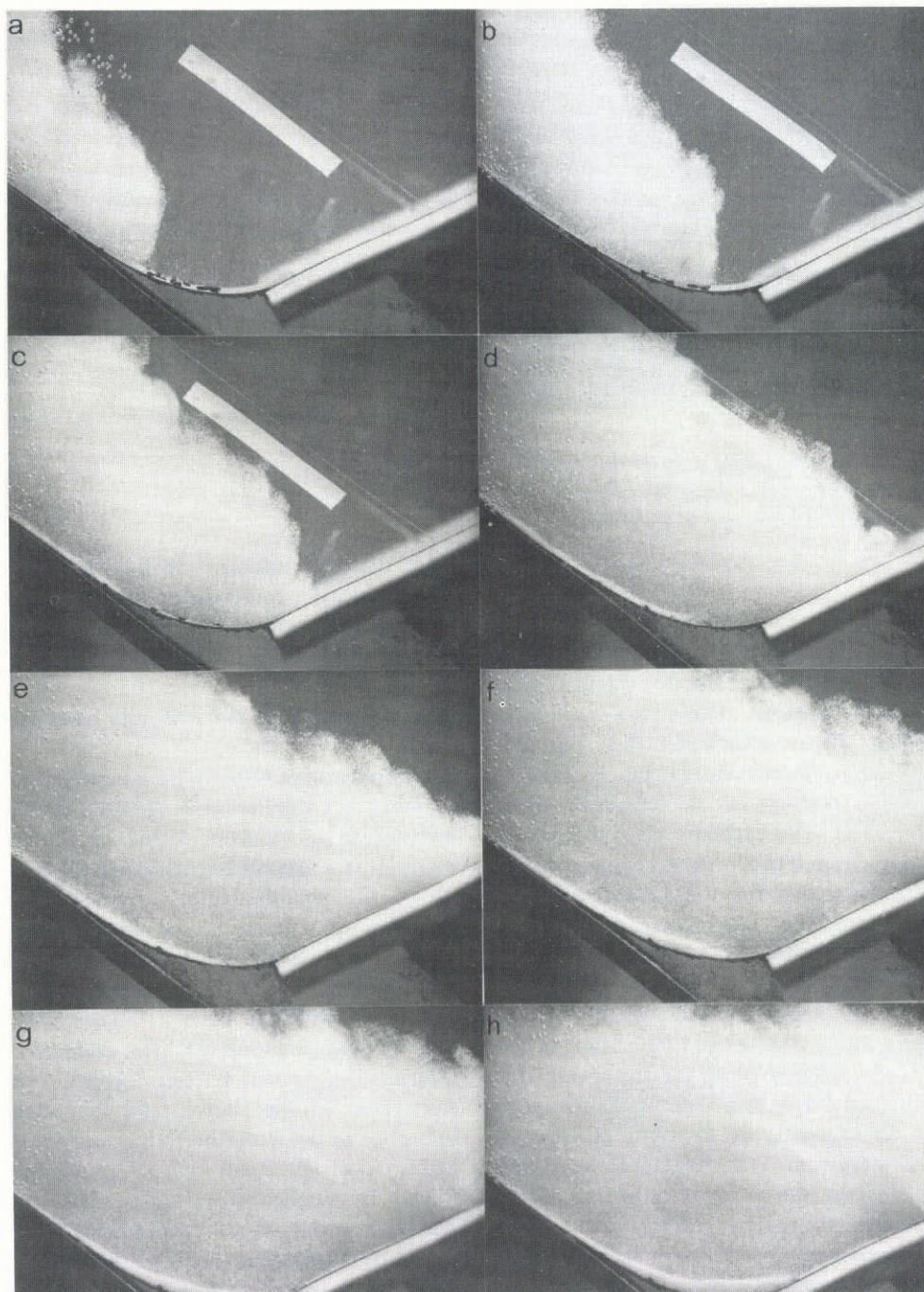
Fig. 12. The passing of an avalanche in the kink zone captured by a high-speed camera (10 frames/s). In frame (c) a dense layer near the bottom appears, which forms the deposit. Wave patterns on its upper boundary can be seen in frame (d). (Photographs by F. Hermann.)
