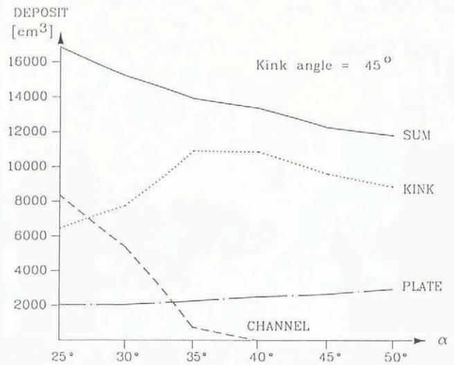
Fig. 13. The measured deposits of seven avalanches versus the chute angle  $\alpha$  at a kink angle  $\beta = 45^\circ$ , split into three parts of the avalanche path (broken lines). The full line is the sum of the deposit. The total material released was approximately  $18000 \text{ cm}^3$ . For  $\alpha < 35^\circ$ , deposition in the steep part of the chute is possible, whereas at higher inclinations this amount of material is concentrated in the kink zone.
