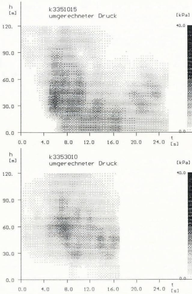
Fig. 19. Time sections of dynamic pressure in positions A (top) and B (bottom), back-calculated as indicated in the text from the data in Figures 14 and 15.
