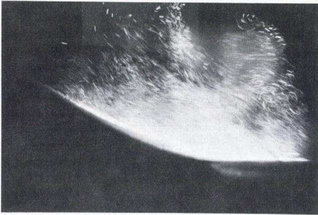
Fig. 10. Particle tracks in the kink zone show the existence of small vortices near the ground and a large one at the upper boundary of the avalanche. (Photograph by F. Hermann.)
