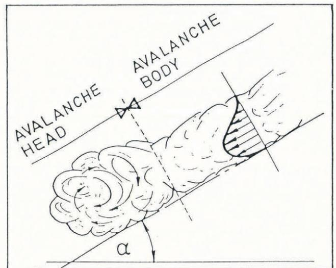
Fig. 5. A typical powder-snow avalanche consisting of a completely turbulent avalanche head and a quasi-stationary avalanche body. A typical velocity profile is shown.
