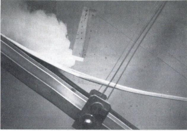
Fig. 18. The sharp front of an avalanche. It corresponds to the density front in Figures 16 or 17.
