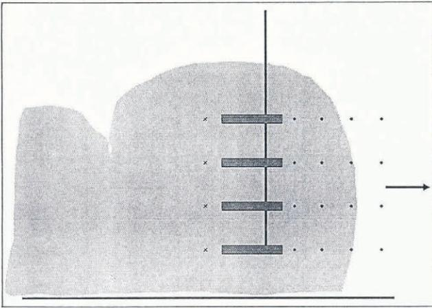
Fig. 6. Time sections are generated with a fixed transducer array when the avalanche moves by, as indicated by the arrow. The position of the actual measuring volume is denoted by ( $\times$ ), while previous positions relative to the moving avalanche are represented by ( $\bullet$ ).
