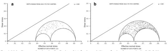
FIG. 4. Mohr diagrams showing the distribution of (*a*) flowing and (*b*) non-flowing fractures in the Sellafield area, UK. None of the fractures are critically stressed at the present-day conditions.
