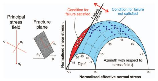
FIG. 1. Critical stress hypothesis (adapted from Barton *et al.*, 1995; Jaeger *et al.*, 2007; Rogers, 2003). The threedimensional Mohr diagram represents the shear stress and normal stress acting along a fracture in response to the *in situ* stress field. The open circles represent fractures experiencing state of stress above the failure criterion and therefore subject to shear failure. The closed circles represent fractures for which the stress state is insufficient to induce shear failure.
