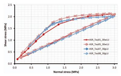
FIG. 8. Shear stress vs. normal stress plot showing prominent hysteresis during the unloading stages of both water and gas injection experiments. The graphs show remarkable similarity in the way shear stress fluctuates with normal stress variations.
