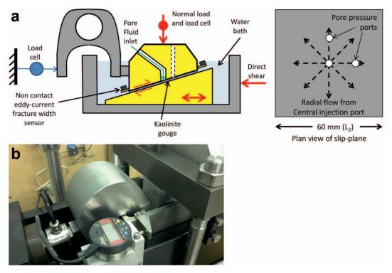
FIG. 5. The angled shear rig (ASR). (*a*) Schematic showing the main components of the apparatus. (*b*) The ASR. The clay gouge sits in between the top and bottom blocks and the pore fluid is injected through an inlet located at the centre of the top block.
