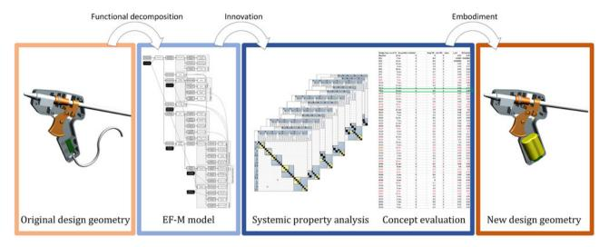
Fig. 6. Visualization of the concept evaluation process; EF-M model containing all variants, DSM derived from the EF-M model, table of 56 concepts and evaluation criteria with the baseline highlighted in blue and the chosen concept in green, renderings of baseline and chosen concept.
