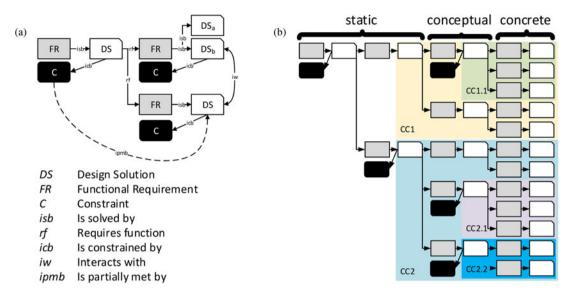
Fig. 1. EF-M modeling: (a) modeling elements, adapted from Johannesson and Claesson (2005) and (b) levels of EF-M tree based on Levandowski et al. (2014) and encapsulation through CC.
