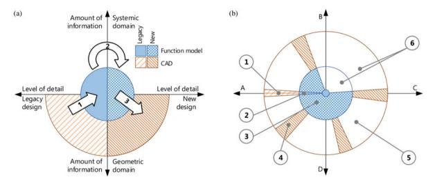
Fig. 7. Design space exploration process using FMs as an intermediate step. (a) Illustrates the steps (1) functional decomposition, (2) innovation, and (3) embodiment to get from legacy to novel design. (b) Provides a top view of the same graph, showing the design space (5) and how it can be explored using function (2, 3) and geometry (1, 4) models.
