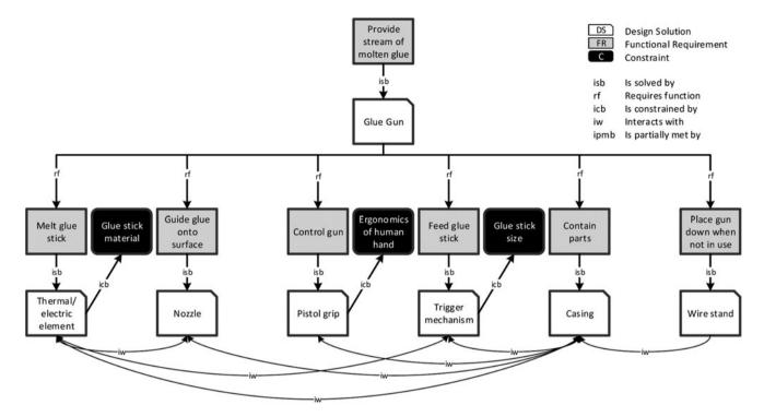
Fig. 2. Initial functional segmentation of the glue gun.
