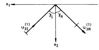
FIGURE 2. Angles of incidence and reflection.
