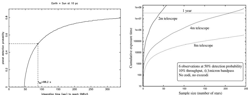
**Figure 3.** Left: Evolution of the planet detection probability (with a signal to noise ratio  $SNR = 5$ ) as a function of exposure time for an Earth-Sun system at 10pc ( $m_V = 5$ ,  $1 mas$  angular diameter,  $100 mas$  maximum angular separation) observed by a 4m telescope. The bandwidth is  $\Delta\lambda = 0.3 \mu m$  and the central wavelength is  $\lambda = 0.5 \mu m$ . Right: Cumulative exposure time required for the survey of a sample of up to 250 stars for ETPs.
