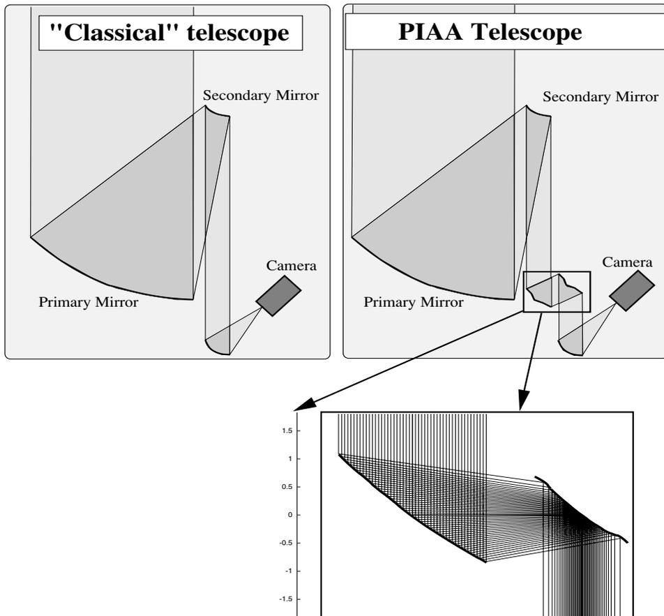
**Figure 1.** Illustration of the PIAA technique (bottom): a collimated unapodized beam can be amplitude-apodized without light loss thanks to 2 aspheric mirrors. The system preserves the flatness of the wavefront of an on-axis source.
