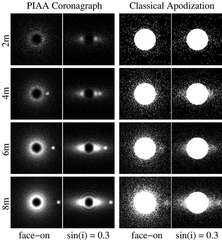
**Figure 4.** Simulated  $0.55 \mu\text{m}$  images of HIP4569 and an hypothetical Earth-type planet at maximum elongation for telescope sizes ranging from 2m to 8m. For each coronagraph/telescope size combination, images were produced in the optimistic face-on case (left) and the inclined  $\sin(i)=0.3$  case (right). See text for details.
