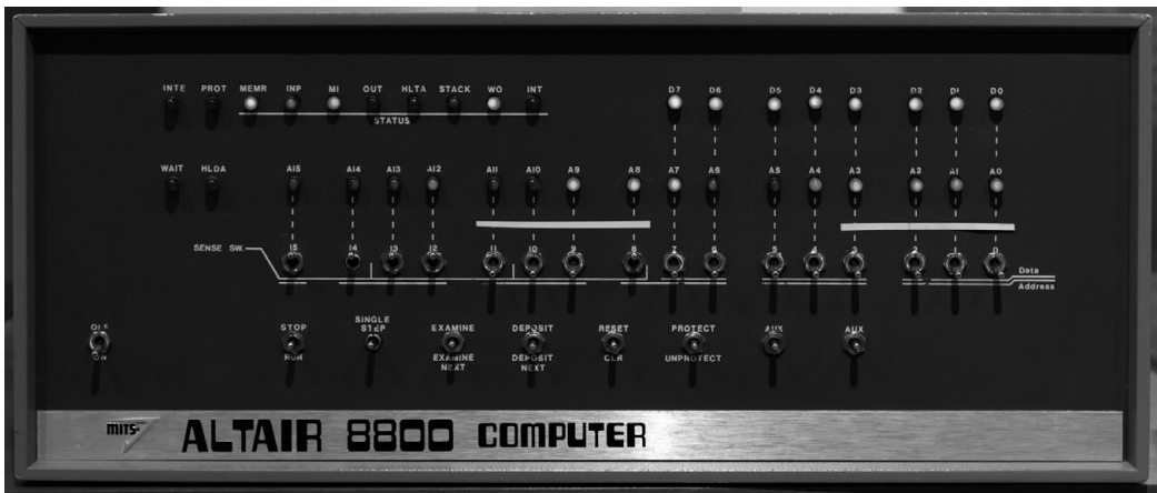
Figure 3.12 Front panel of Altair 8800, showing the status lights, a row of switches for specifying addresses and entering data and a row of control switches. (Source: Living Computers Museum, Photo by Michael Dunn, 97 CC-BY 2.0)
