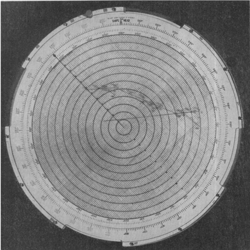
*Fig. 1. The compass-datum computer. The relative bearing (outer) ring may be turned to set ship's head to any desired point on the compass course or bearing scale and then clamped. The compass scale is fixed to the plotting surface. The graticule with its pointer is on a disk which may be turned independently of either bearing scale. The computer, being circular, may be held with either ship's-head or north (000°) upwards, according to preference.*
