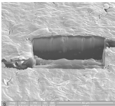
FIG. 1. SEM image of a polymer – metal particle composite illustrating cracking due to sample heating.
