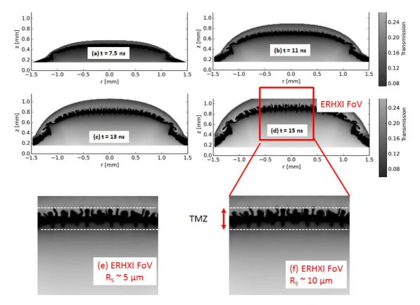
**Figure 10.** (a) to (d) Postprocessed radiographs of RTI multimode evolution with a titanium backlighter according to ERHXI spatial resolution of  $10 \,\mu$ m. (e) and (f) Comparison of ERHXI field of view with spacial resolution of  $5 \,\mu$ m and  $10 \,\mu$ m. The tips of the spikes are better resolved in (e). The turbulent mixing zone width is defined as the average distance between the RTI spike and bubbles.
