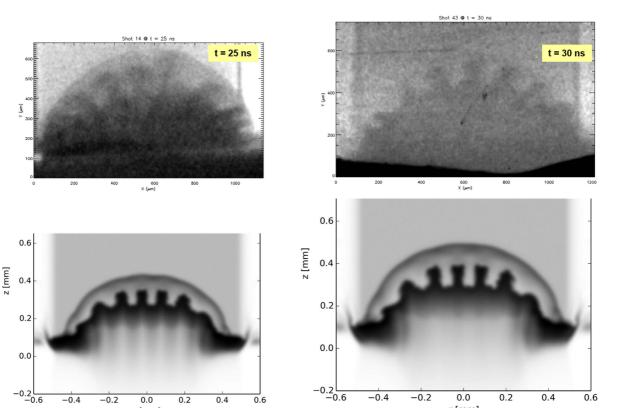
Figure 6. Comparison of experimental (first row) and postprocessed FLASH hydrodynamics simulations (second row).
