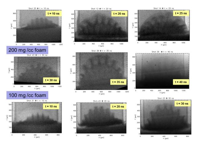
Figure 5. Experimental radiographs acquired on imaging plate (IP) on LULI2000. Acquisition times correspond to the Pico2000 delay relative to the main drive. The first RTI data were acquired on Shot 22 and Shot 23.
