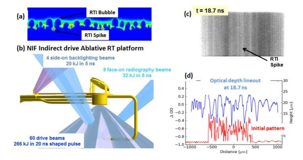
**Figure 2.** (a) FCI2 calculations showing bubble-merger regime for indirect-drive experiments on NIF<sup>[10, 31, 32]</sup>. (b) Experimental configuration with simultaneous face-on and side-on radiographies. (c) Face-on radiograph acquired at t = 18.7 ns. (d) The lineout extracted from (c) shows how the initial broadband pattern (in red) has evolved into 6 main bubbles as a result of the bubble-competition regime.
