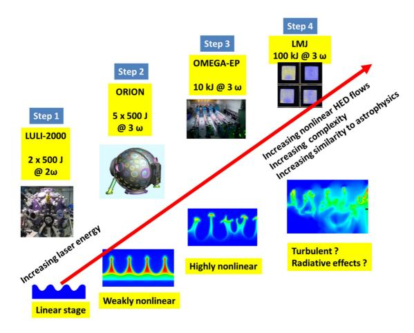
Figure 3. Envisioned laser plasma experiments within the TurboHEDP project. The higher the laser energy and the longer the laser drive, the more nonlinear HED flows become, with the final goal to create on LMJ turbulent HED flows. Typical side-on views of ablative RTI single-mode and multi-mode simulations<sup>[10, 36]</sup> are shown to illustrate the increasing level of nonlinearity of the flows expected on each facility.
