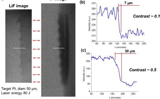
Figure 8. Comparison of LiF and IP images for the same (undriven) modulated target. The spatial resolution is estimated to be 7 µm in the LiF case, compared to 30 µm with IP.
