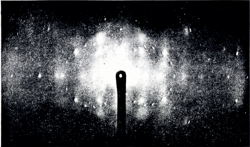
Fig. 1. Laue photograph of ice, using unfiltered radiation from a copper target; incident beam 1 mm. diameter, exposure time one hour; temperature about -5^{\circ} C. Crystal orientation: [00.1] axis vertical, incident beam nearly parallel to (11.0) plane. Cylindrical film. Showing sharp Laue spots and diffuse thermal vibration pattern superimposed. Note the strong 00.2 thermal reflection a little way above the central spot, although the (00.2) plane is horizontal
