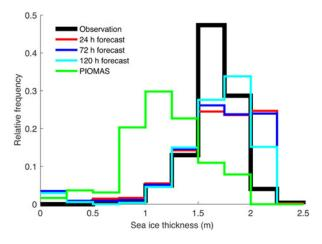
**Fig. 6.** Histogram of sea-ice thickness of each data during *Xuelong*'s transit through the trans-Arctic Passage from 2 August to 19 August. The ASPeCt observations aboard *Xuelong* are shown in black. The 24, 72, and 120 hour forecasts are shown in red, blue and cyan, respectively. PIOMAS data are shown in green.
