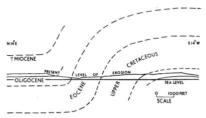
TEXT-FIG. 1.-The Isle of Wight monoclinal fold form (based on part of Section No. 2, Sheet 47 of the Horizontal Sections of the Geological Survey).
