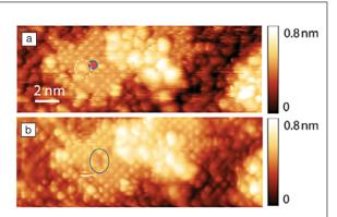
In situ mapping of La<sub>0.625</sub>Ca<sub>0.375</sub>MnO<sub>3</sub> surface morphology before (a) and after (b) an electrochemical reaction. The white and blue circles mark the formation of an oxygen vacancy. Reprinted with permission from Appl. Phys. Lett. 106 (2015), 143107. © 2015 AIP Publishing LLC.
