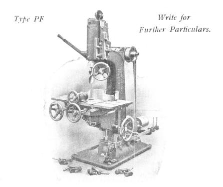
For boring, drilling, and recessing the bosses of propellers, etc.; half lapping the laminations; recessing and drilling the spars, etc.
