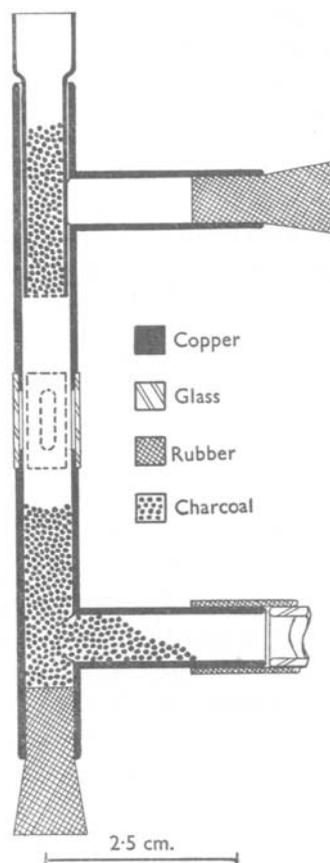
Text-fig. 1. Ultra-microscope cell, section normal to axis of microscope. Position of observation window shown dotted.
