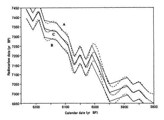
Fig. 1. Section of the <sup>14</sup>C calibration curve.  $\_$  = linear interpolations between data points, ---- = cubic spline interpolations; C = interpolated measurements; A and B =  $\pm$  1  $\sigma$  errors on the measurements
