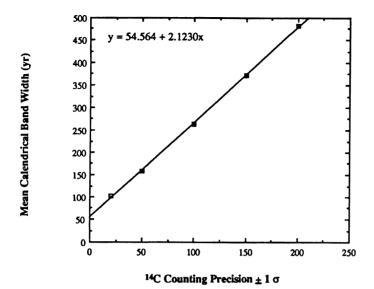
Fig. 5. Mean calendrical band width as a function of <sup>14</sup>C precision
