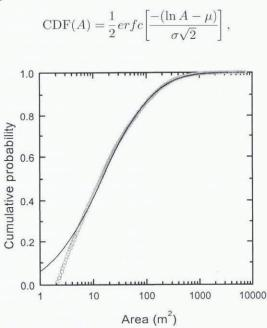
Fig. 4. Cumulative melt-pond size distribution for > 28 000 ponds taken from the 31 July 1994 photographs. The squares are the observations and the curve is the two parameter lognormal best-fit distribution.
