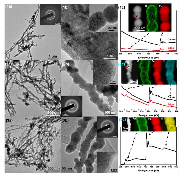
**Figure 1.** TEM image (a) and HRTEM image (b) of Fe-Fe<sub>x</sub>O<sub>y</sub> NWs. Inset in (a) and (b) is the corresponding ED pattern and low mag. TEM image, respectively. (c) Position-dependent EELS spectra recorded from edge (red) and central (black) positions of NWs. HAADF images and elemental mapping of O and Fe, are shown in upper part of panel.
