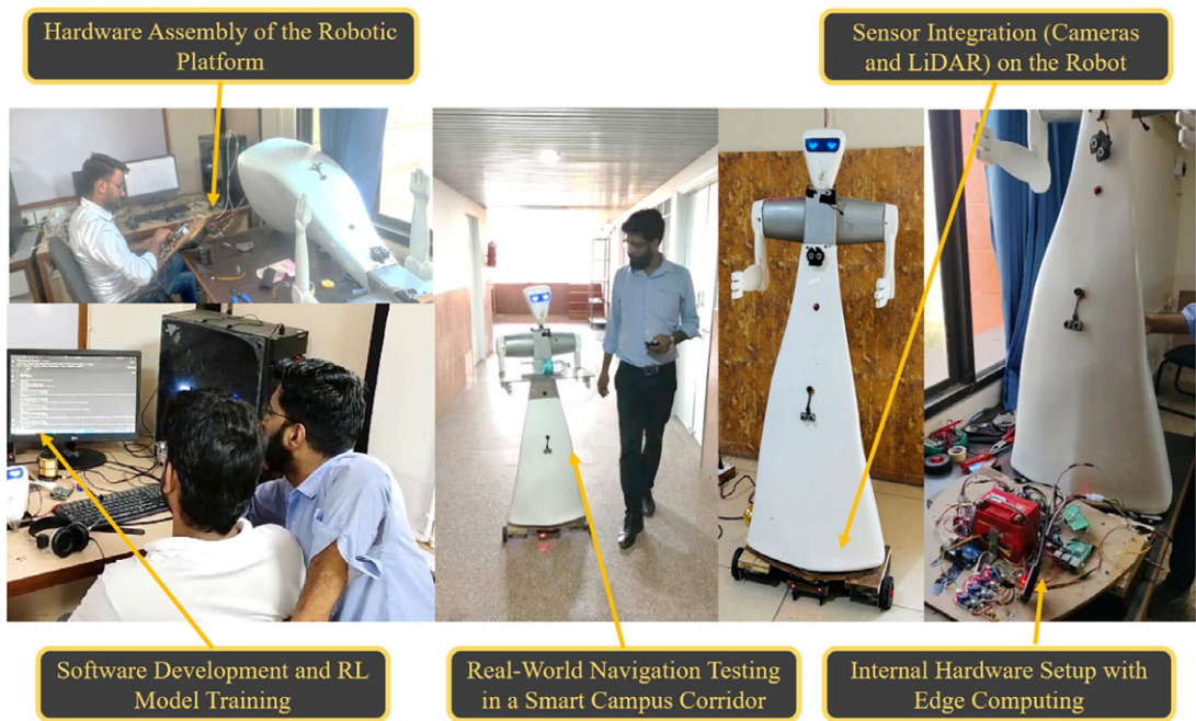
Figure 8. Real-time deployment of the suggested robotic navigation framework. The figure indicates key milestones including hardware integration of the robot platform, sensor onboarding (LiDAR and cameras), reinforcement learning model training, and internal edge computing setup.
