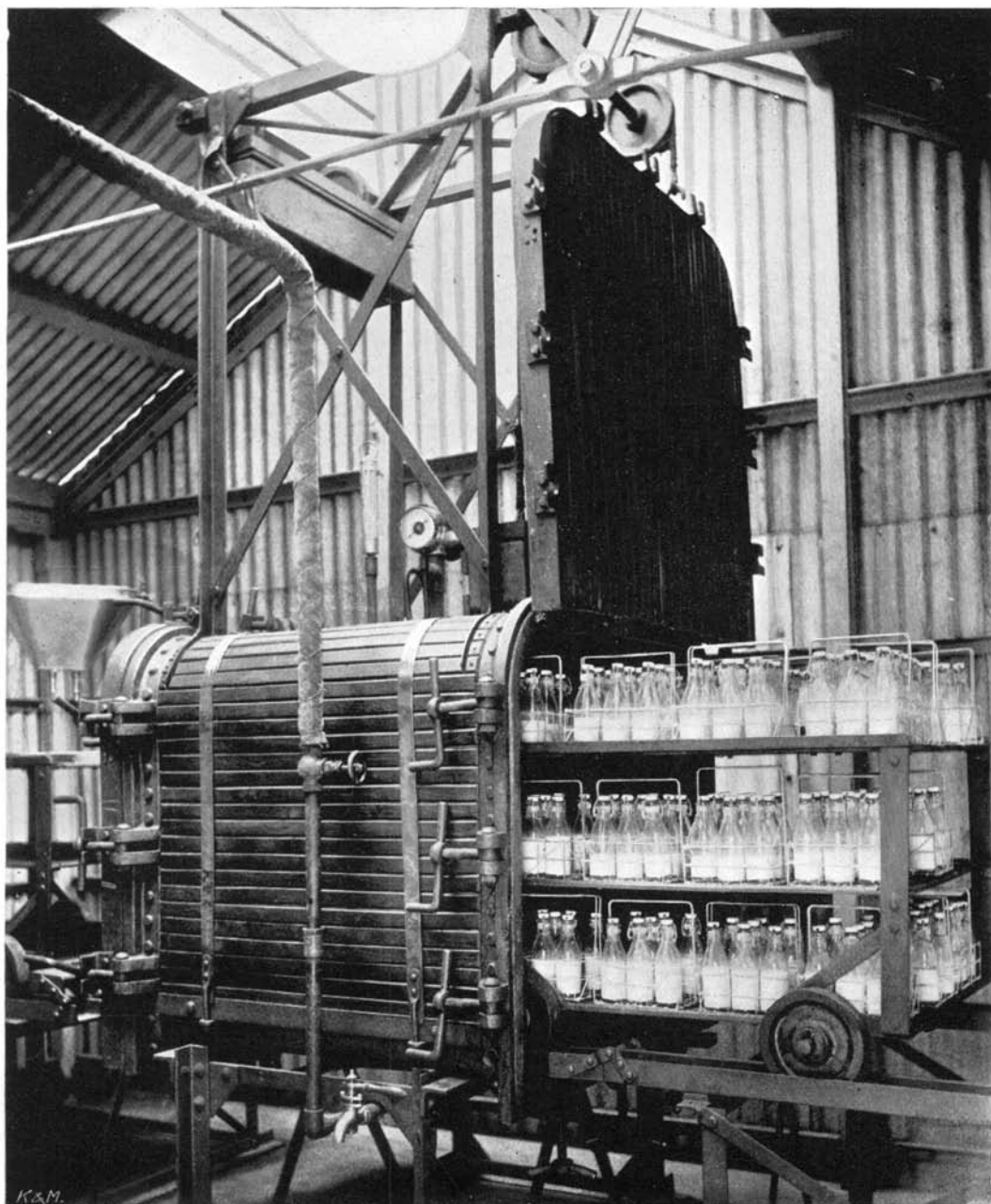
Infants' Milk Depot, Battersea. Interior of sterilising room, showing steriliser with loaded trolley.
