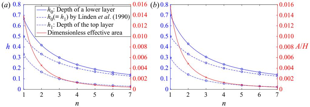
Figure 5. The reduction in the dimensionless layer depth with the number of interfaces. The depths of lower layers  $h_0$  and top layer  $h_1$  are plotted from the solution of (6.7) and (6.9). The Linden *et al.* (1990) prediction, (1.1), is displayed for comparison. The red line, with scale given on the right-hand side vertical axis, plots the variation of  $A/H$  with  $n$ : (a)  $\mathcal{A} = 1$ ; (b)  $\mathcal{A} = 1.46$ , the aspect ratio used in the experiments of Cooper & Hunt (2010).
