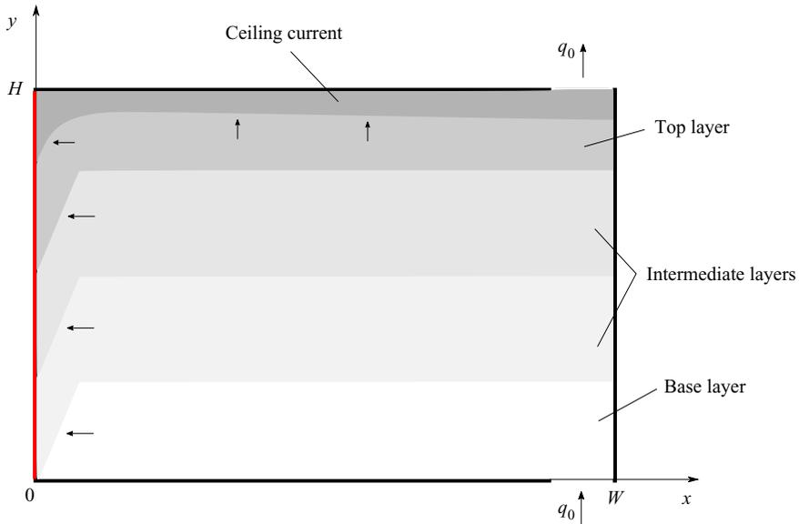
Figure 1. Schematic showing a vertical section through a box with height  $H$  and width  $W$ , coordinate system and stable stratification established by a turbulent wall plume from a vertically distributed buoyancy source on the wall (left). The stratification induces a volume flow rate  $q_0$  through openings in the base and top. The darkening grey scale indicates regions of increasing buoyancy.
