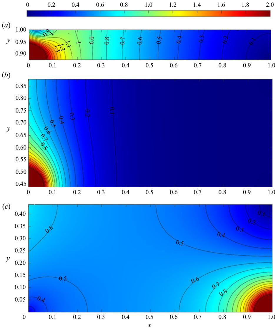
Figure 7. Colour map and contours showing the distribution of dimensionless velocity magnitude  $U(x, y)$  corresponding to the streamline pattern for  $\mathcal{A} = 1$  and  $n = 2$  shown in figure 6(b). (a) Top layer. (b) Intermediate layer. (c) Base layer. The velocity associated with each colour is indicated on the horizontal scale above (a).
