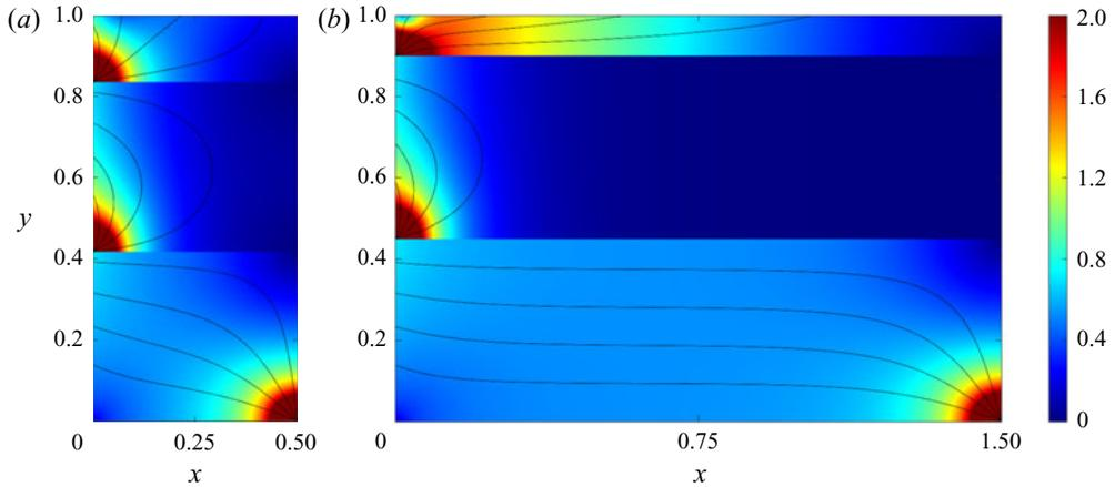
Figure 9. Colour map of dimensionless velocity magnitude  $U(x, y)$  overlain with streamline pattern for the  $n = 2$  stratification; (a)  $\mathcal{A} = 0.5$ , (b)  $\mathcal{A} = 1.5$ . The step between two adjacent streamlines is  $\Delta\psi = 0.05$ . The vertical colour bar indicates the magnitude of the dimensionless velocity.
