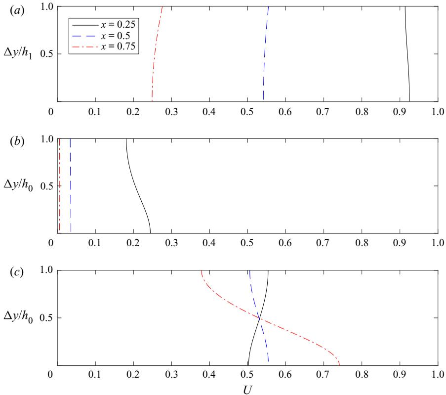
Figure 8. Vertical profiles of dimensionless velocity magnitude  $U$  at a quarter ( $x = 0.25$ ), a half ( $x = 0.5$ ) and three quarters ( $x = 0.75$ ) of the box width from the wall plume;  $\mathcal{A} = 1$ ,  $n = 2$ . (a) Top, (b) intermediate and (c) base layer. Here,  $\Delta y$  denotes the vertical distance from the base of each layer.
