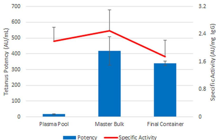
**Fig. 2.** Tetanus potency and specific activity of tetanus immune globulin during manufacture by the caprylate/chromatography process (TIG-C). Data are expressed as the mean  $\pm$  s.d. A marginal dilution may occur from Master Bulk to Final container to target potency/ml of product.
