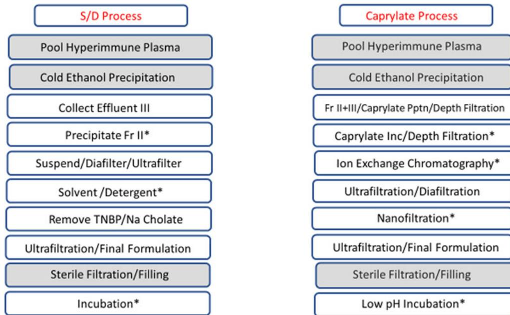
**Fig. 1.** Flow diagrams for the solvent/detergent (S/D) and caprylate/chromatography processes. The grey bars denote steps that are common to both processes and the asterisks (\*) mark steps that have been validated to deactivate and/or remove blood-borne pathogens. Fr, fraction; TNBP, tri-n-butyl phosphate; Pptn, precipitation; Inc, incubation. This figure was modified from Woznichak *et al.* [24].
