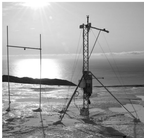
Fig. 5. Photograph of AWS1 at 330 m a.s.l. on Sørbreen, 2 October 2008. The mast is 5 m high and stands freely on the ice (photograph by K. Breili).
