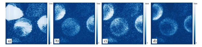
**Figure 2.** Comparison of images taken with 300keV and a readout out speed of 1000fps under constant TEM settings in the different pnCCD operation modes: a) The high electron dose causes overflowing pixels in the Normal mode. b) More TEM electrons can be collected in the pixels in the HCHC mode. c) The AB mode prevents overflowing pixels. d) The XPLUS mode prevents overflowing pixels while increasing the number of collectable TEM electrons.
