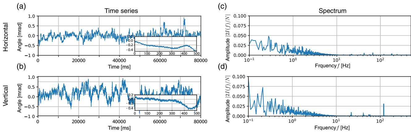
**Figure 4.** (a), (b) Time series of 1 kHz non-amplified beam pointing angle at focus in horizontal and vertical directions, derived from the far-field mode captured by camera 2 and the near-field mode captured by camera 3. (c), (d) The amplitude  $|2I(f)/N|$  of the discrete Fourier transform  $I(f)$  of the time series (a) and (b), respectively, highlighting the dominant components below 10 Hz.
