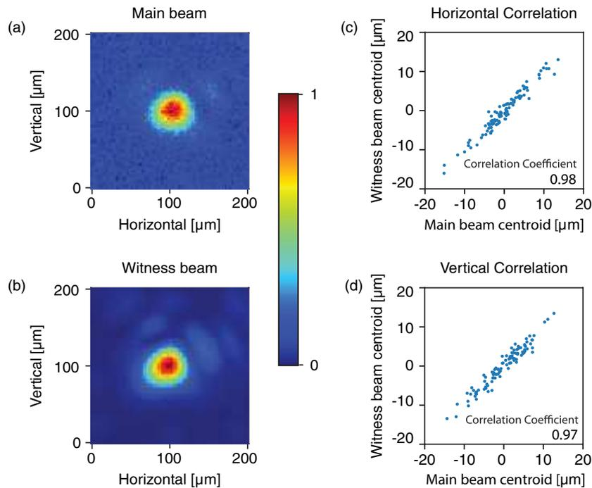
**Figure 2.** A single-shot transverse mode profile of the amplified beam captured by (a) camera 1 (mode imager) and (b) camera 2 (witness beam). (c), (d) Correlation of 100 consecutive high-power shots (at 1 Hz) of the main beam and witness beam centroids in horizontal and vertical direction, respectively.
