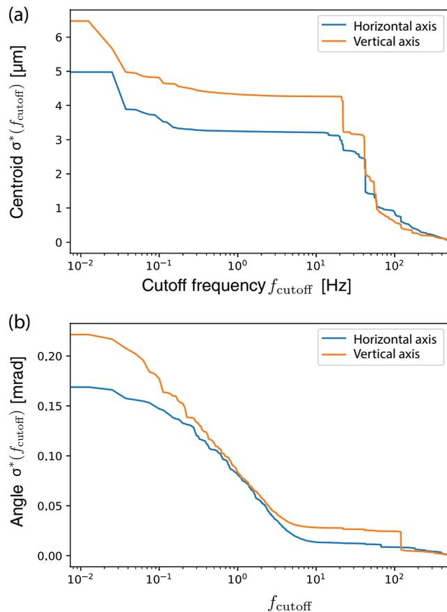
**Figure 5.** The standard deviation  $\sigma^*$  of (a) the centroid fluctuations and (b) the angle fluctuations, with only frequencies above  $f_{\text{cutoff}}$  included in the standard deviation calculation. This representation of the spectral content is a complementary way to interpret the Fourier transforms of the time series in Figures 3 and 4.
