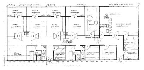
*Figure 9:* European ward block in Oshakati hospital. Drawing 'Okatana hospital, Ovamboland, Plan of European ward block'. Source: Drawing Archive in Ministry of Works, Transport and Communication.
