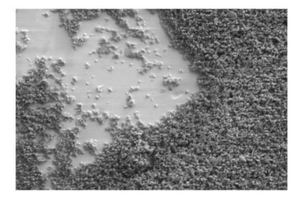
**Figure 1** Secondary electron image of a  $30 \times 20 \,\mu\text{m}^2$  area on grain dispersion mount CG. The region in the centre contains well dispersed grains. Grains in such regions were used for single grain analysis. The region on the right is entirely covered with grains. Such regions were chosen for raster ion imaging.
