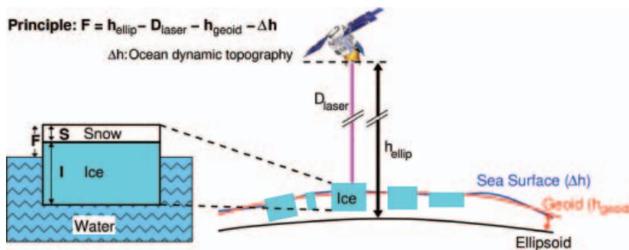
**Fig. 2.** Schematic diagrams showing the interrelation of ice freeboard,  $F$ , snow depth,  $S$ , and sea-ice thickness,  $I$ , (left) and an artist's view of ICESat above the three involved surfaces: reference ellipsoid, geoid and sea surface (right).
