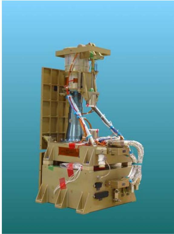
**Figure 7.** One of two redundant framing cameras.
