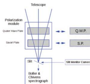
**Figure 1.** Optical design of the system Telescope - Polarizer Module - Spectrograph
