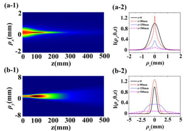
**Figure 5.** Normalized intensity distribution of an NMGC partially coherent beam on propagation in free space (a-1) in  $\rho_x$ - $z$  plane, and (b-1) in  $\rho_y$ - $z$  plane with  $x_0 = 0$  and  $M = 5$  and the corresponding cross-line.
