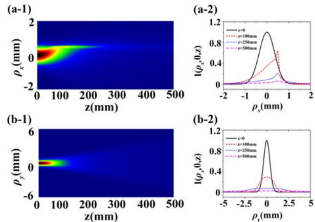
**Figure 6.** Normalized intensity distribution of an NMGC partially coherent beam on propagation in free space (a-1) in  $\rho_x$ - $z$  plane, and (b-1) in  $\rho_y$ - $z$  plane with  $x_0 = \sigma_0$  and  $M = 20$  and the corresponding cross-line.
