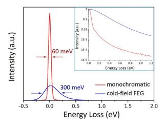
Figure 1. Comparison of the ZLP taken on the Nion UltraSTEM with and without the monochromator. The main figure is normalized to the integrated intensity, while the inset is normalized to the maximum intensity of the ZLP.
