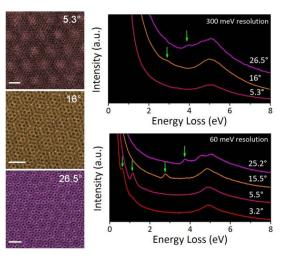
Figure 2. (Left) Experimental ADF images of twisted bilayer graphene with different misorientation angles. Scale bars: 1 nm. (Right) Low-loss EEL spectra of the TBG acquired using the Nion UltraSTEM with and without the monochromator. The misorientation angles are labeled on each spectrum.
